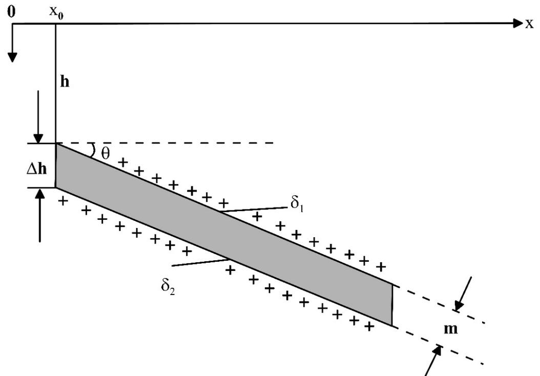
**Figure 1.** The source geometry for the 2D dipping layer/bed.
