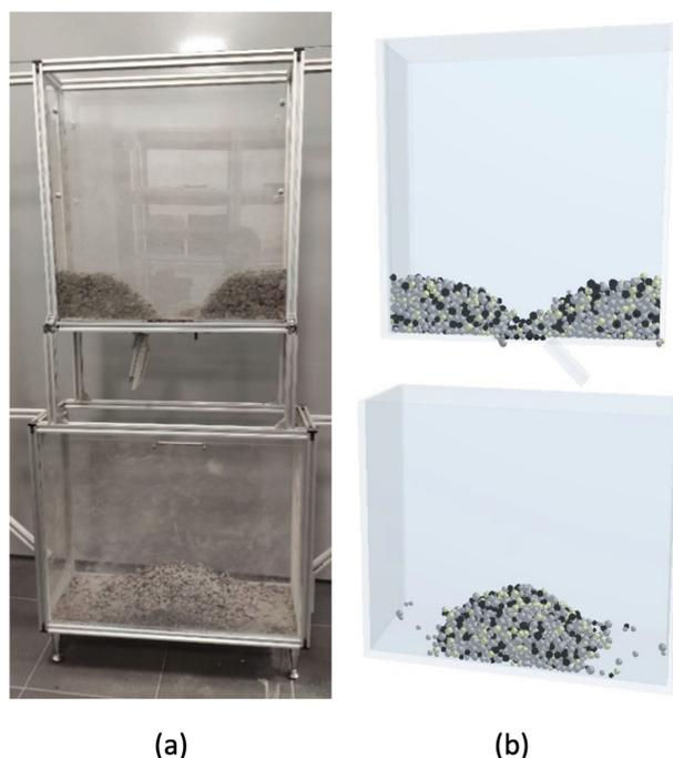
**Figure 8.** Calibration test stand: (a) performed experiment and (b) simulated experiment.
