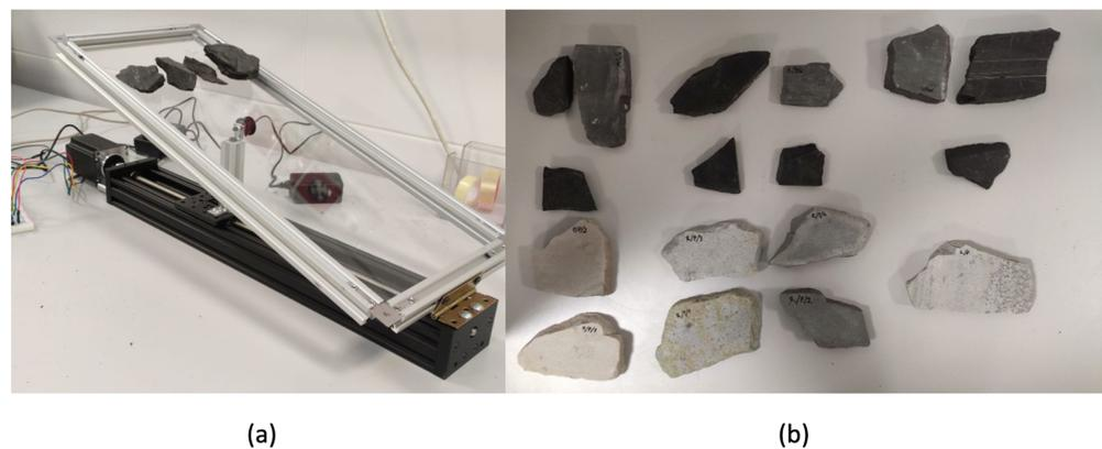
**Figure 4.** Measuring static friction: (a) incline plane and (b) flat surface samples used as liners.
