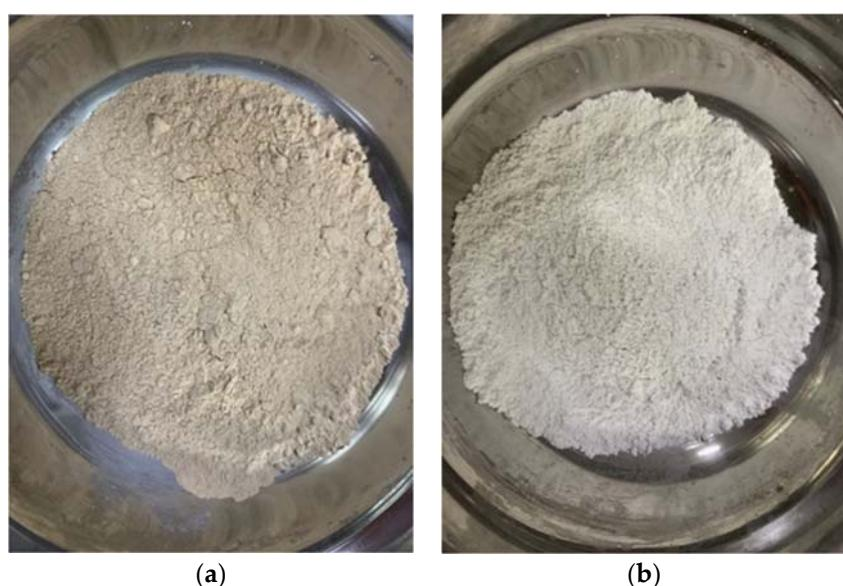
**Figure 2.** Ordinary kaolin (a) and ordinary metakaolin (b).
