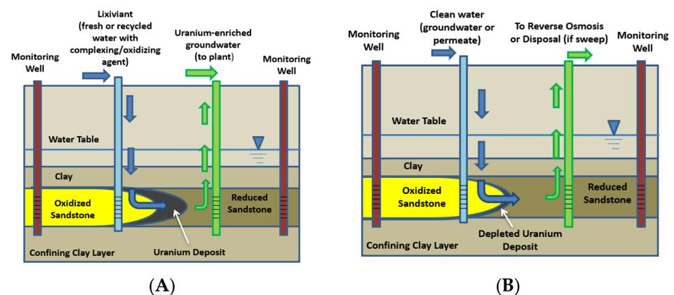
**Figure 2.** A conceptual model of the (A) production and (B) restoration phases of uranium ISR.
