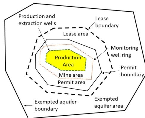
**Figure 3.** Nomenclature and relationships of the different “area types” associated with a uranium in-situ recovery mine.
