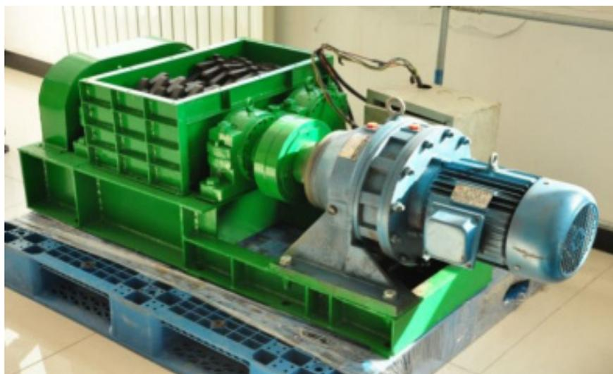
**Figure 5.** ZKB-II shear breaker.
