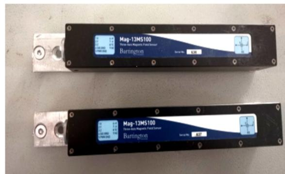
**Figure 3.** Magnetic field information collector.
