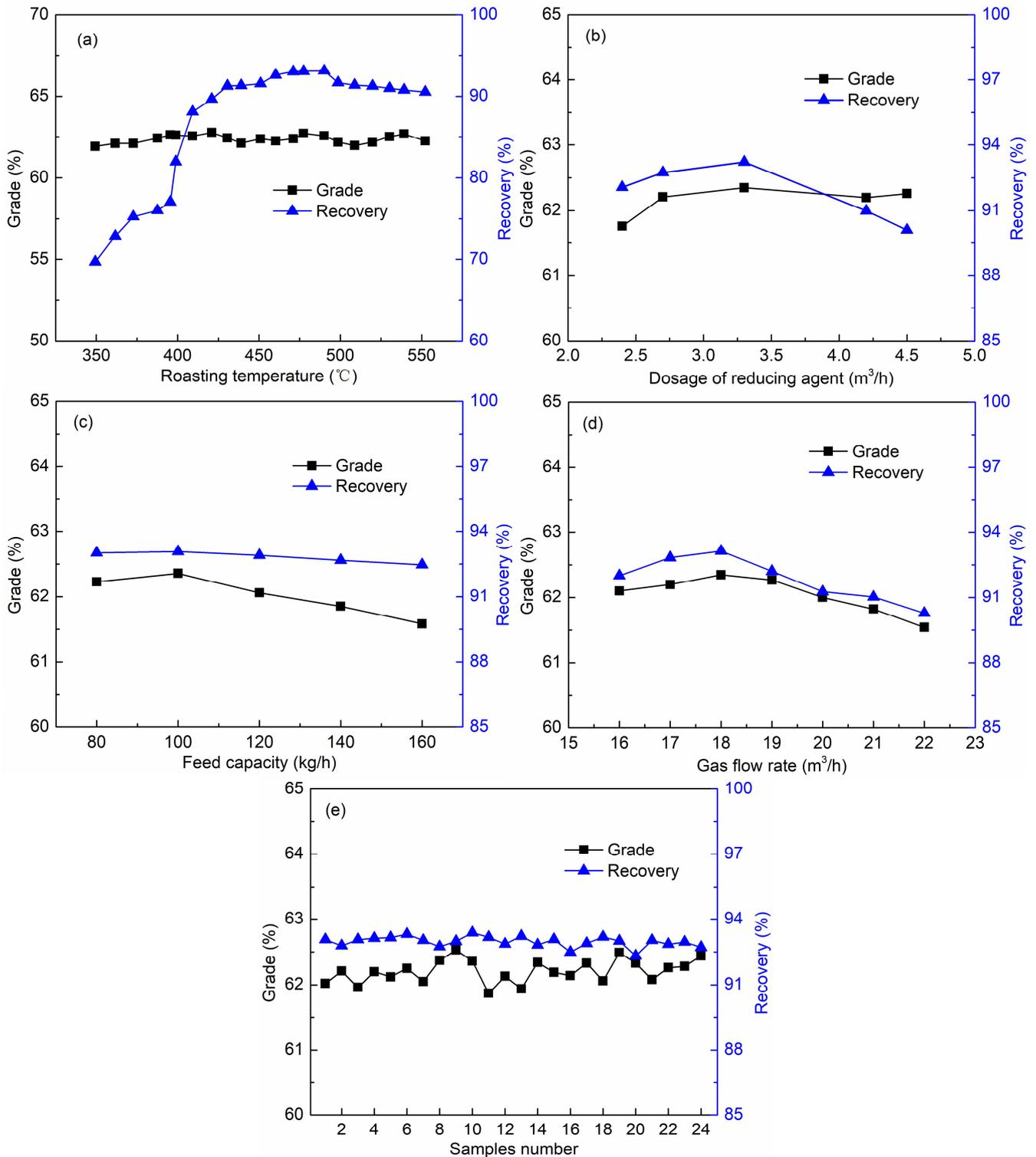
**Figure 3.** Effects of roasting conditions on Fe grade and recovery of magnetic concentrate. (a) roasting temperature; (b) reducing agent dosage; (c) feeding capacity; (d) gas flow rate; (e) stable running test.
