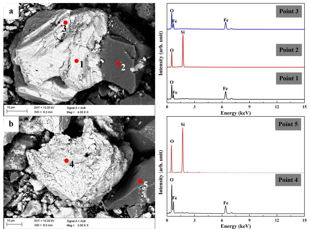
**Figure 7.** Micromorphology analysis of different products (a) pre-concentration concentrate; (b) roasted samples.
