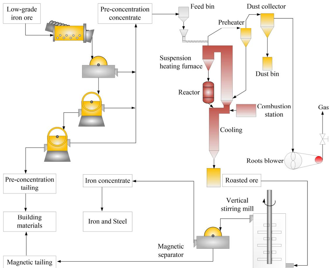
Figure 2. Schematic diagram of comprehensive utilization of low-grade iron ore.
