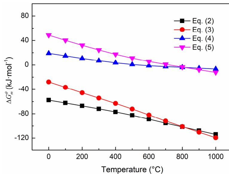
**Figure 5.** Thermodynamics analysis of reduction reaction Equations (2)–(5).
