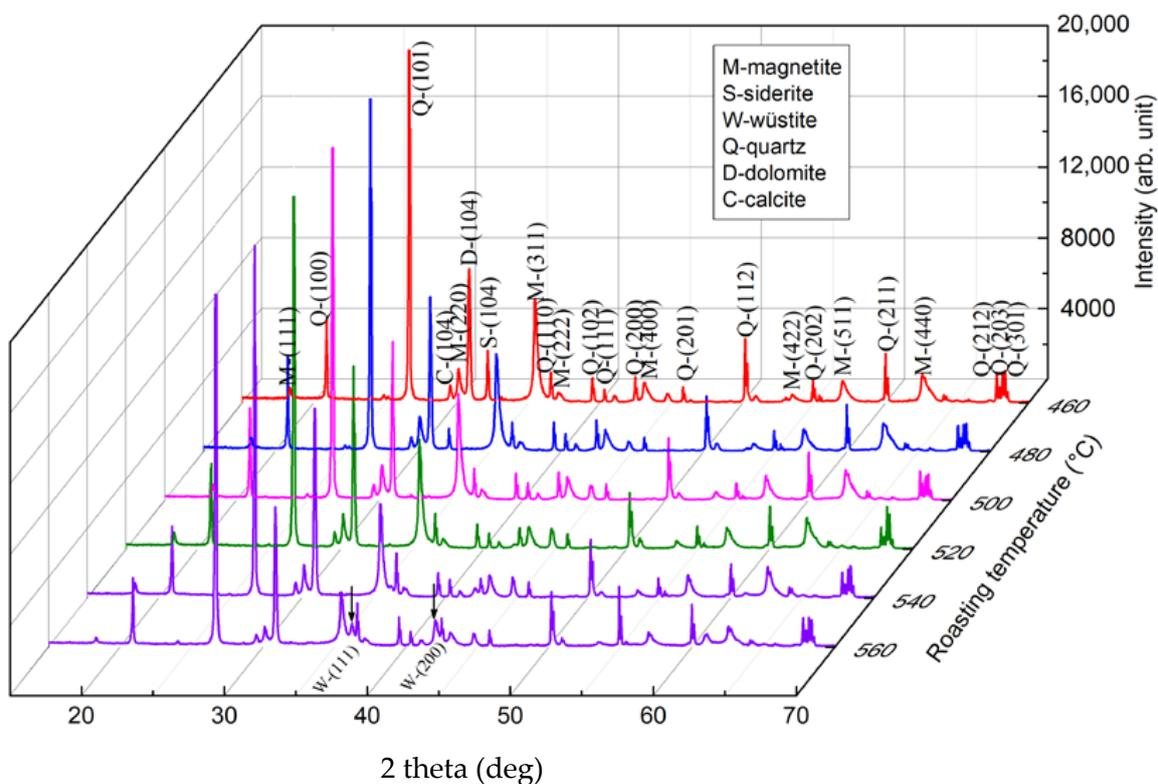
Figure 4. XRD analysis of the roasted products at different roasting temperatures.
