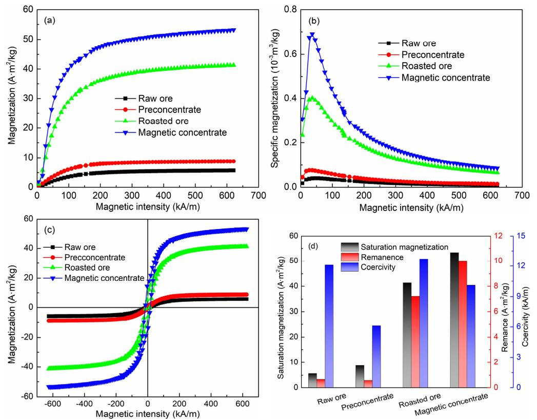
**Figure 6.** Magnetism properties of different products (a) initial magnetization curves; (b) Specific susceptibility curves; (c) hysteresis loops; (d) magnetism parameters.
