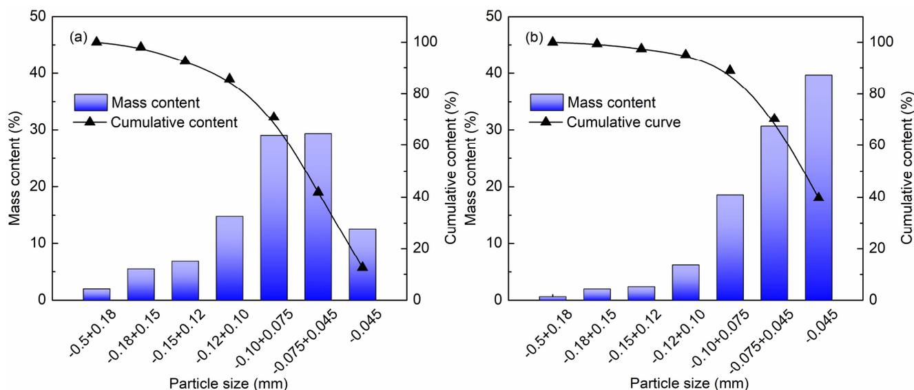
**Figure 8.** Particle size analysis of tailings (a) pre-concentration tailing; (b) magnetic tailing.
