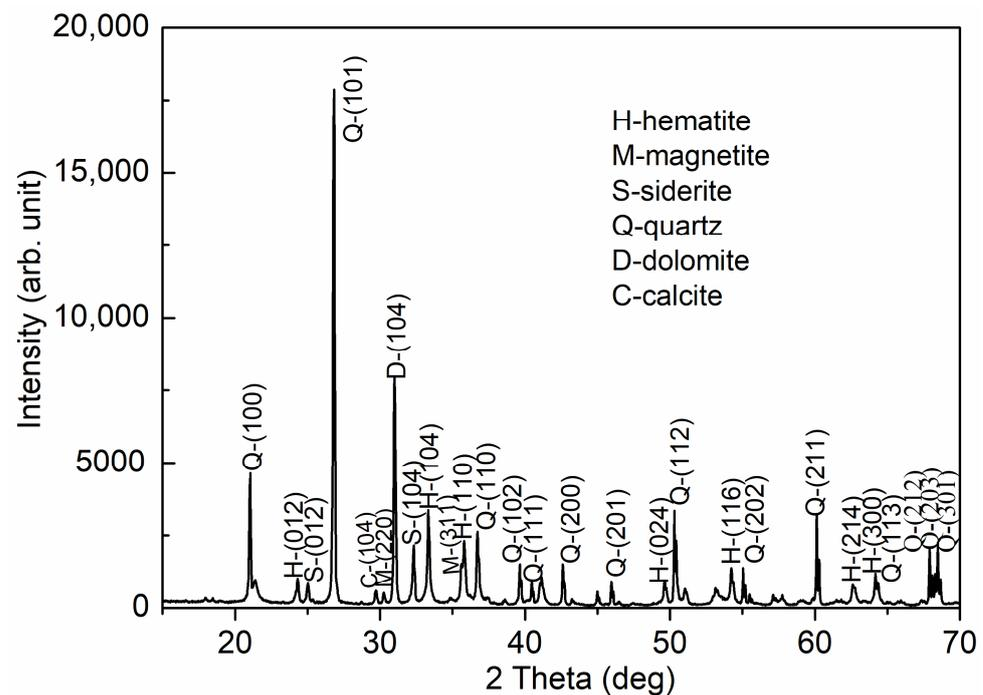
Figure 1. XRD analysis of raw ore.
