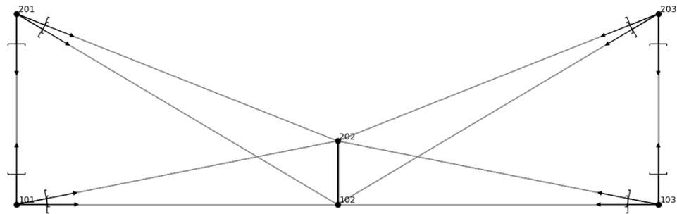
Figure 2. Six-points control network segment.
