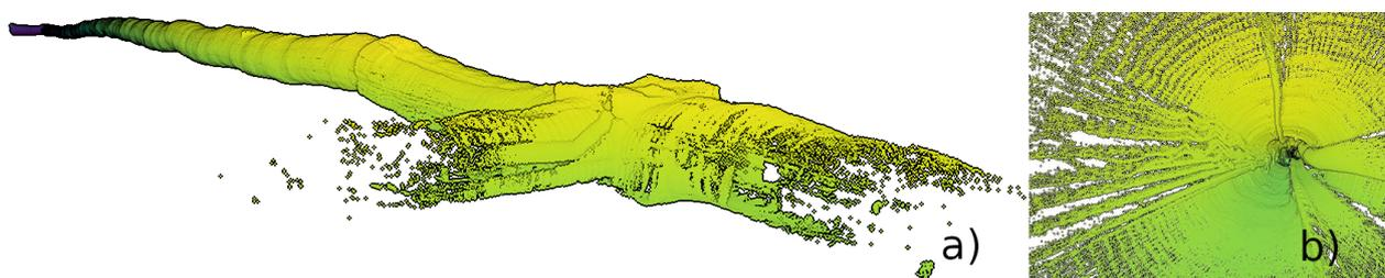
**Figure 6.** Point cloud of a mine segment. (a) Whole cloud (outside view), (b) view from inside, along the tunnel.
