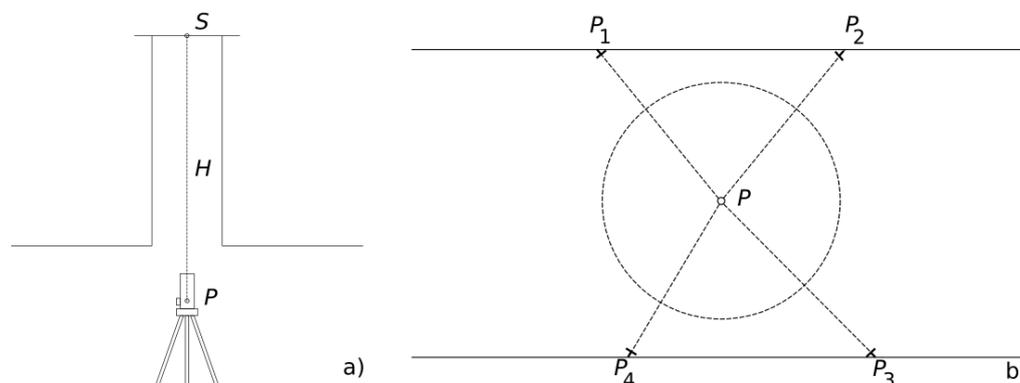
**Figure 5.** Network connection via a vertical shaft. (a) Vertical projection, (b) horizontal projection.
