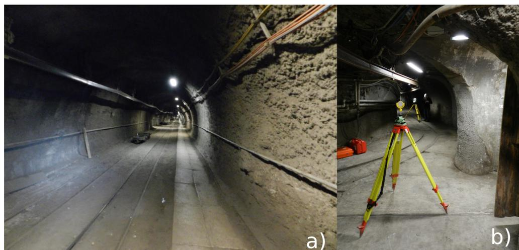
**Figure 1.** Traversing through underground tunnels in Velenje Coal Mine. (a) Straight segment, (b) retro-reflector and total station.
