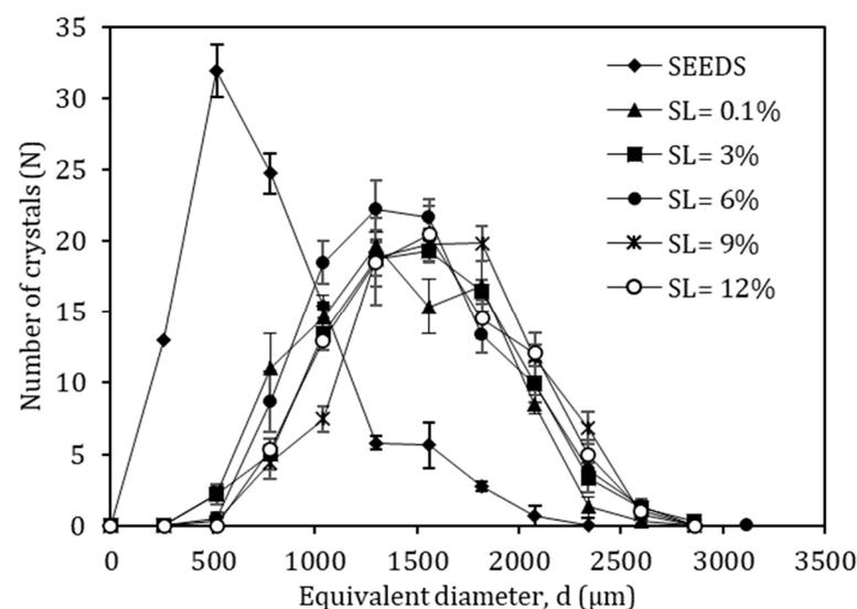
Figure 14. Effect of ice seed loading on ice product size.
