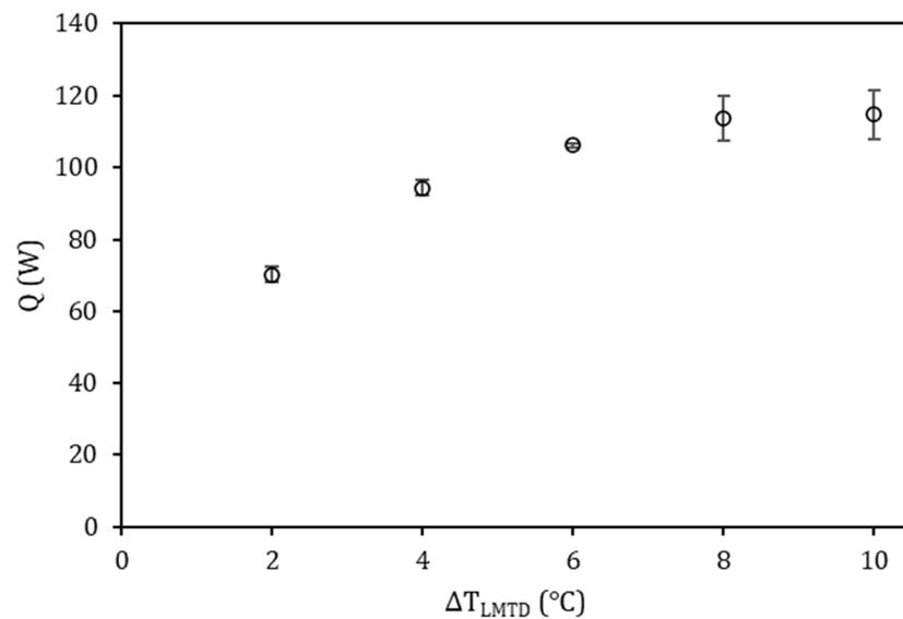
Figure 6. Effect of  $\Delta T_{LMTD}$  on heat transfer rate (Q).
