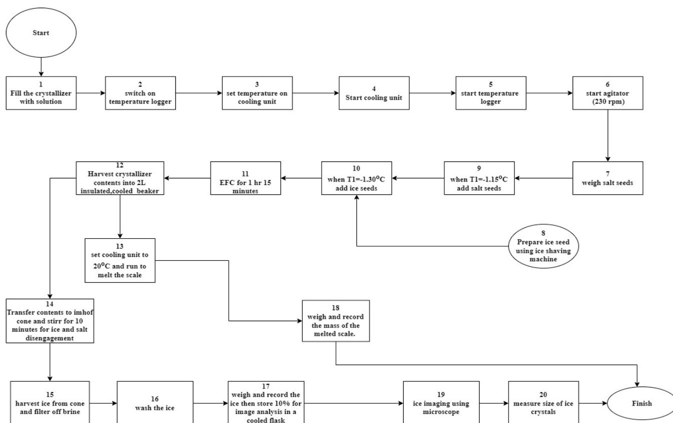
Figure 4. Experimental procedure flow chart.
