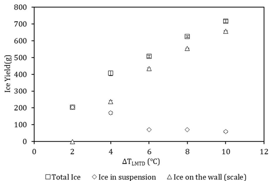
**Figure 5.** Effect of  $\Delta T_{LMTD}$  on total ice yield.
