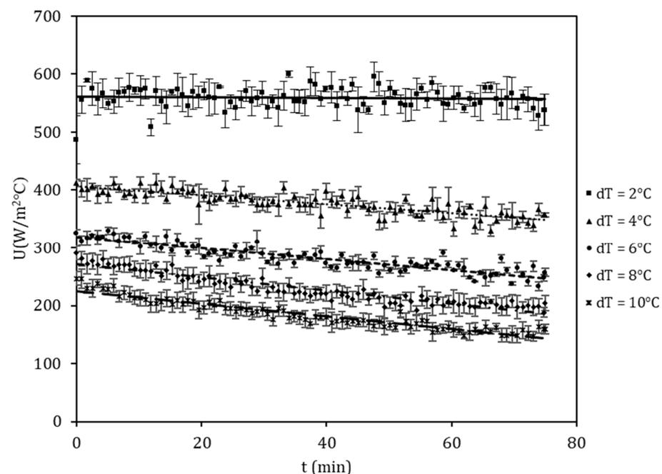
Figure 7. Effect of  $\Delta T_{LMTD}$  on overall heat transfer coefficient (U).
