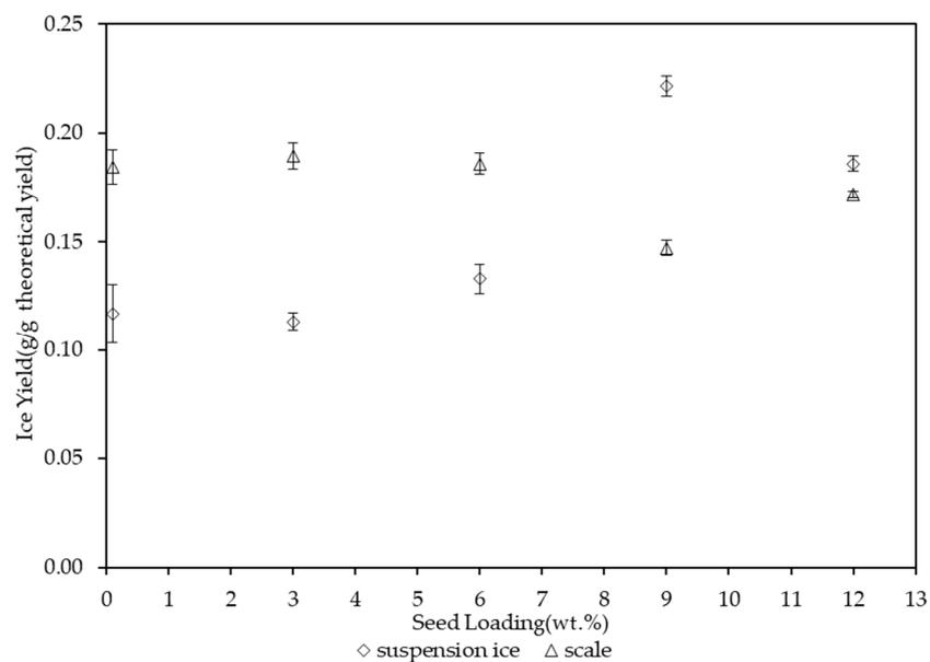
**Figure 10.** Effect of seed loading on suspension and scale ice yield.
