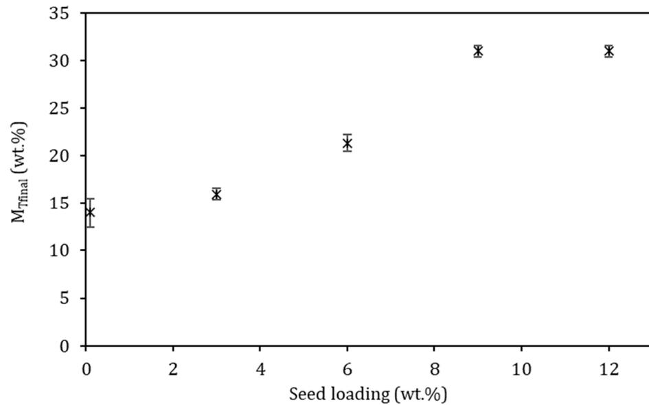
Figure 11. Effect of seed loading ( $M_{T0}$ ) on final magma density ( $M_{Tfinal}$ ).
