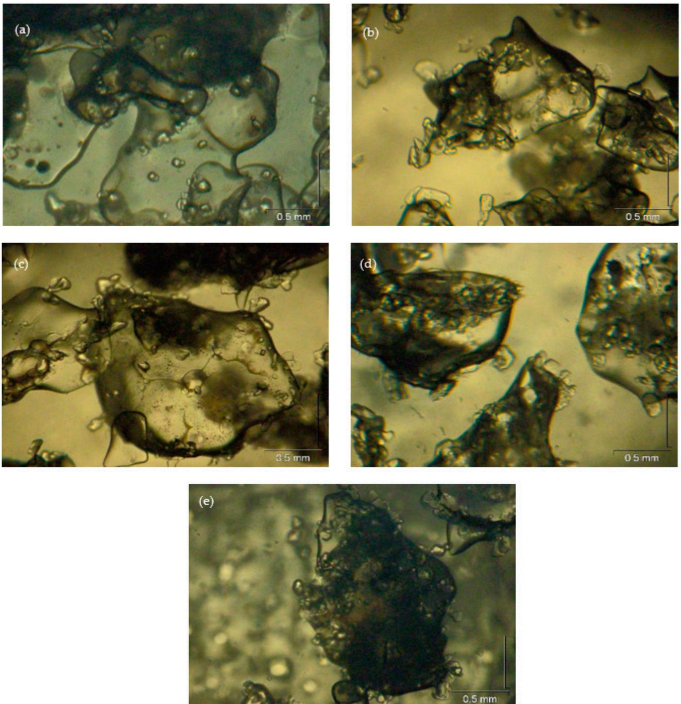
**Figure 15.** Typical ice product at SL = 0.1 (a), 3 (b), 6 (c), 9 (d) and 12 wt% (e).
