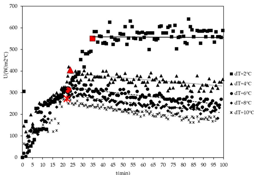
**Figure 8.** Effect of  $\Delta T_{LMTD}$  on overall heat transfer coefficient ( $U$ ), including pre-seeding time interval.
