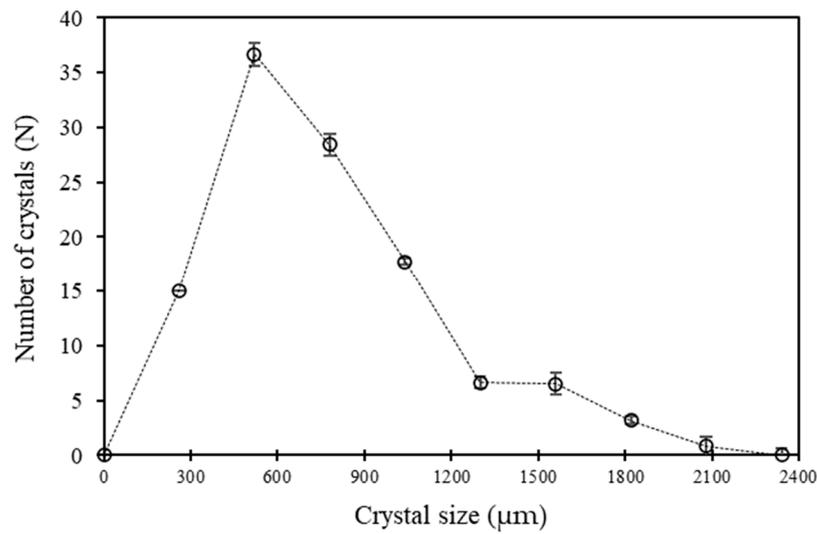
**Figure 2.** Crystal size distribution of the ice seeds formed from the ice shaving machine.
