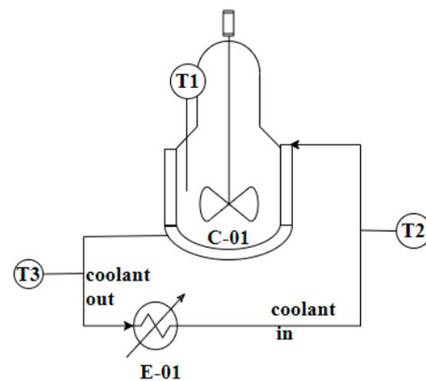
**Figure 1.** Schematic of batch crystallizer setup.
