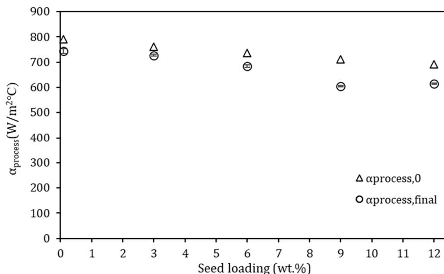
**Figure 13.** Effect of seed loading on process side heat transfer coefficient.
