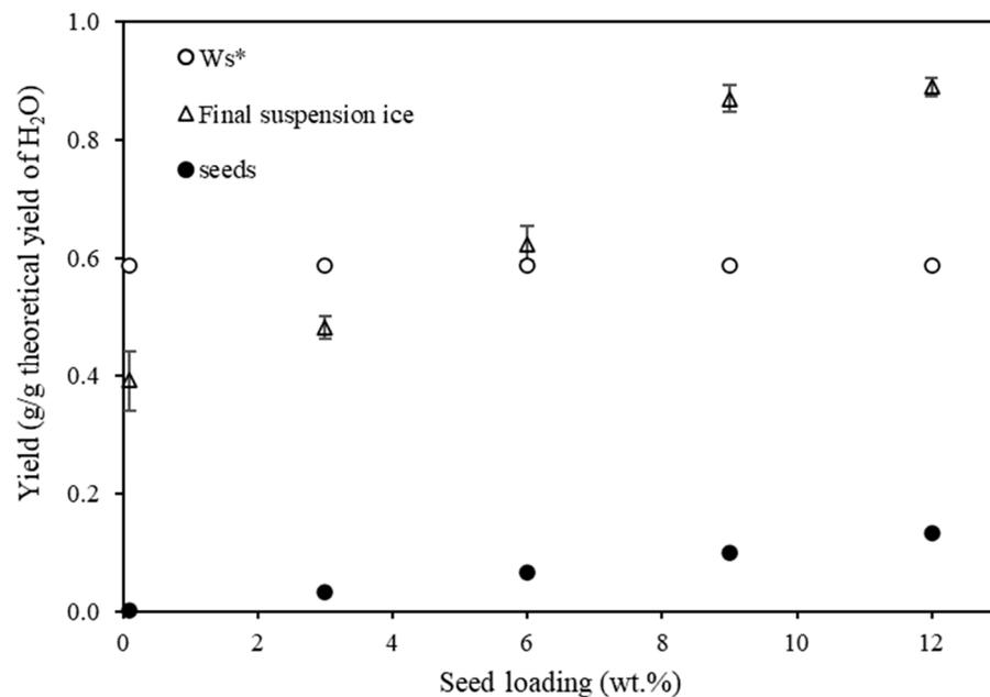
**Figure 16.** Effect of seed loading on final suspension ice and critical seed loading ( $W_s^*$ ).
