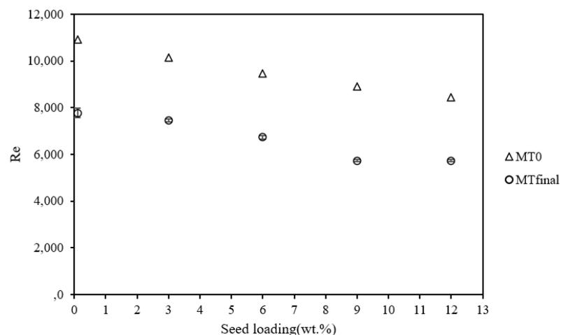
Figure 12. Effect of seed loading on Reynolds number.
