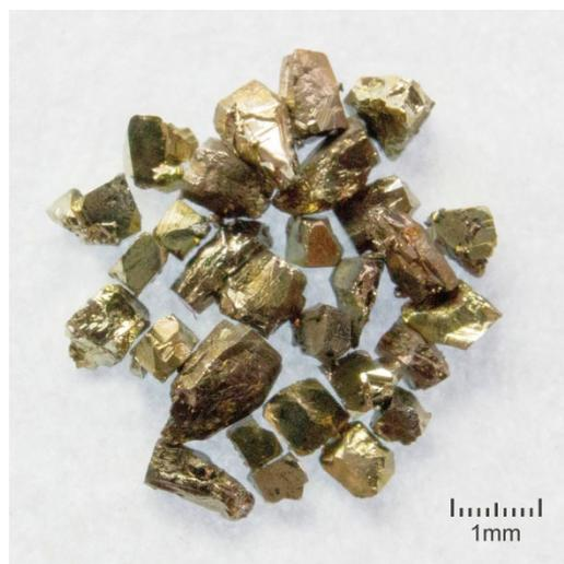
**Figure 1.** Crystals of associated pyrite and pyrrhotite displaying a prevailing crystal habit (synthesis conditions—400 °C, 1 kbar, 10 %  $NH_4Cl$  solution).
