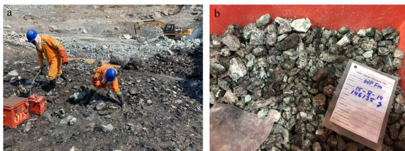
**Figure 4.** (a) Miners use hammers and chisels to extract emeralds from the rock in the reaction zone; (b) The collected emeralds were in a secure box. Photo by Xiangjie Xiao.
