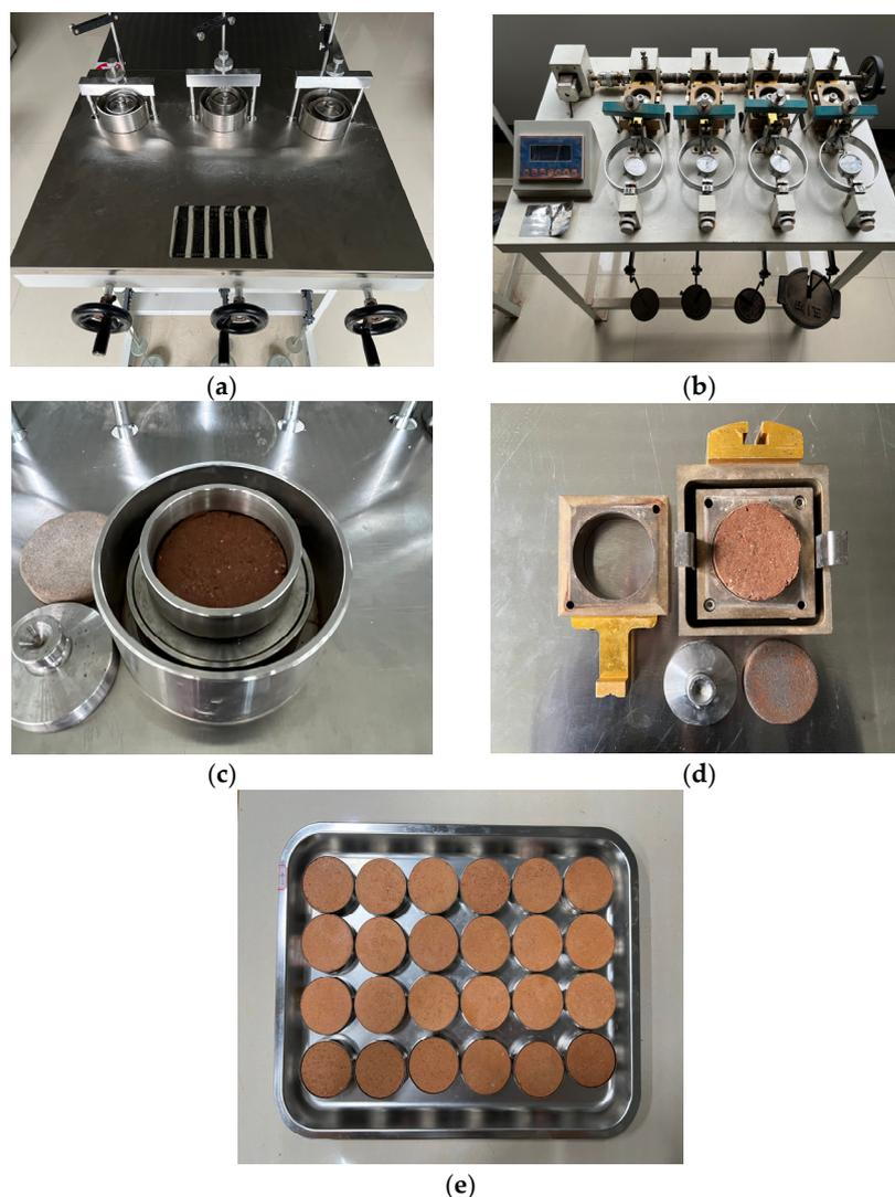
**Figure 2.** The experimental apparatus and specimens. (a) Consolidation apparatus; (b) Direct shear apparatus; (c) Chamber of consolidation apparatus; (d) Chamber of direct shear apparatus; (e) Specimens.
