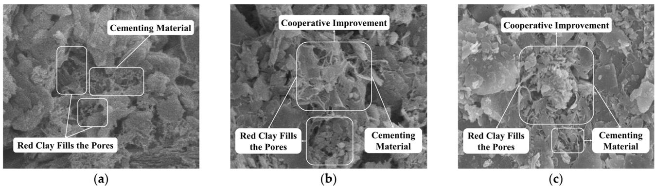
**Figure 13.** Microstructure diagrams of phyllite soil compositely improved with lime and red clay (the SEM images of (a,b) are magnified 30,000 times; the SEM image of (c) is magnified 25,000 times). (a)  $\lambda = 20\% + \eta = 3\%$ ; (b)  $\lambda = 40\% + \eta = 3\%$ ; (c)  $\lambda = 40\% + \eta = 5\%$ .
