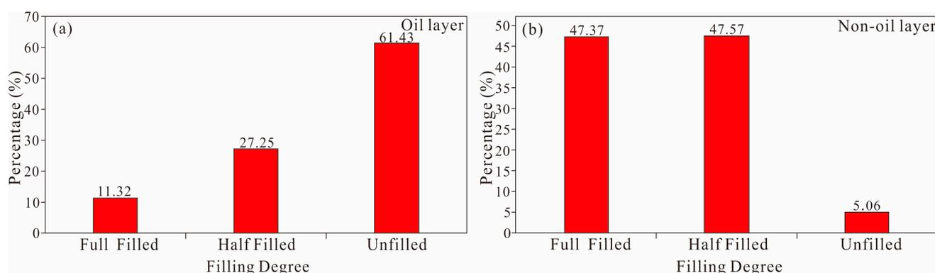
**Figure 8.** Core fracture filling degree distribution histograms. (a) Histogram of distribution of oil layer core filling degree; (b) histogram of distribution of non-oil layer core filling degree.
