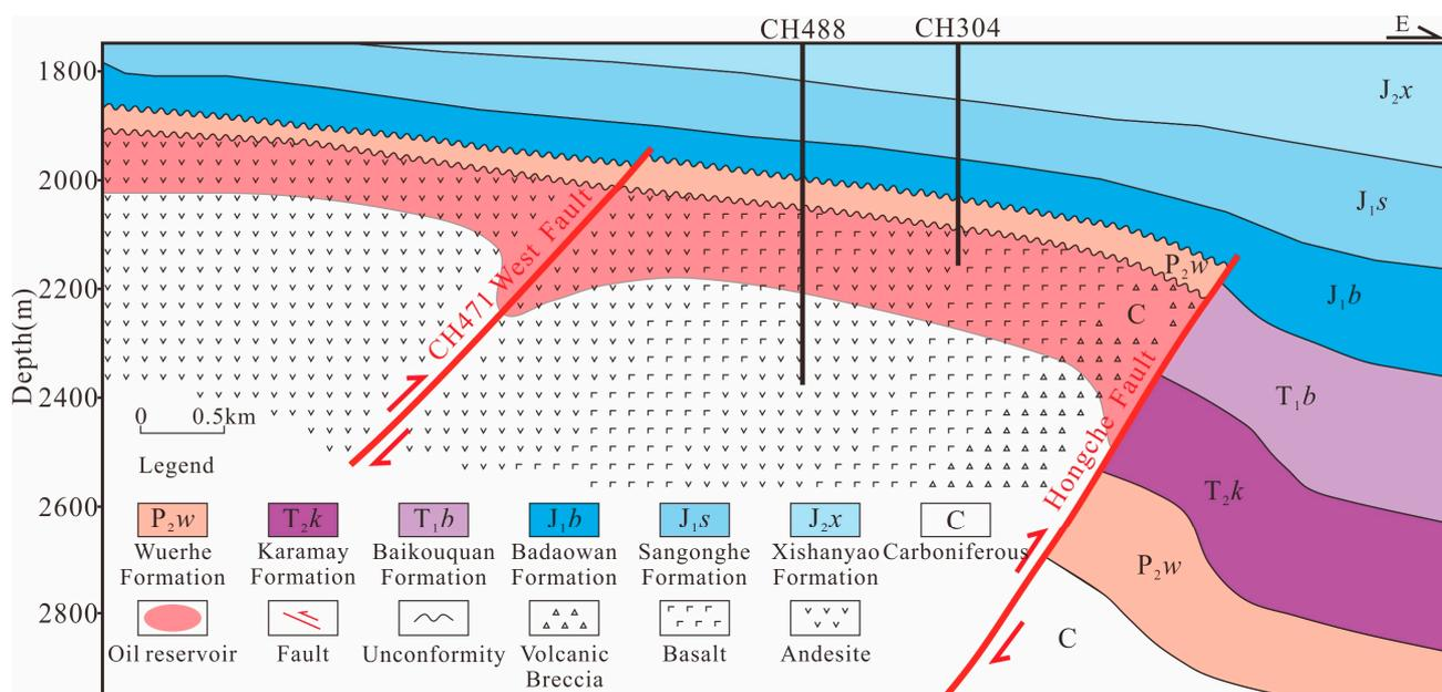
**Figure 2.** Schematic diagram of E-W strike section in the study area.
