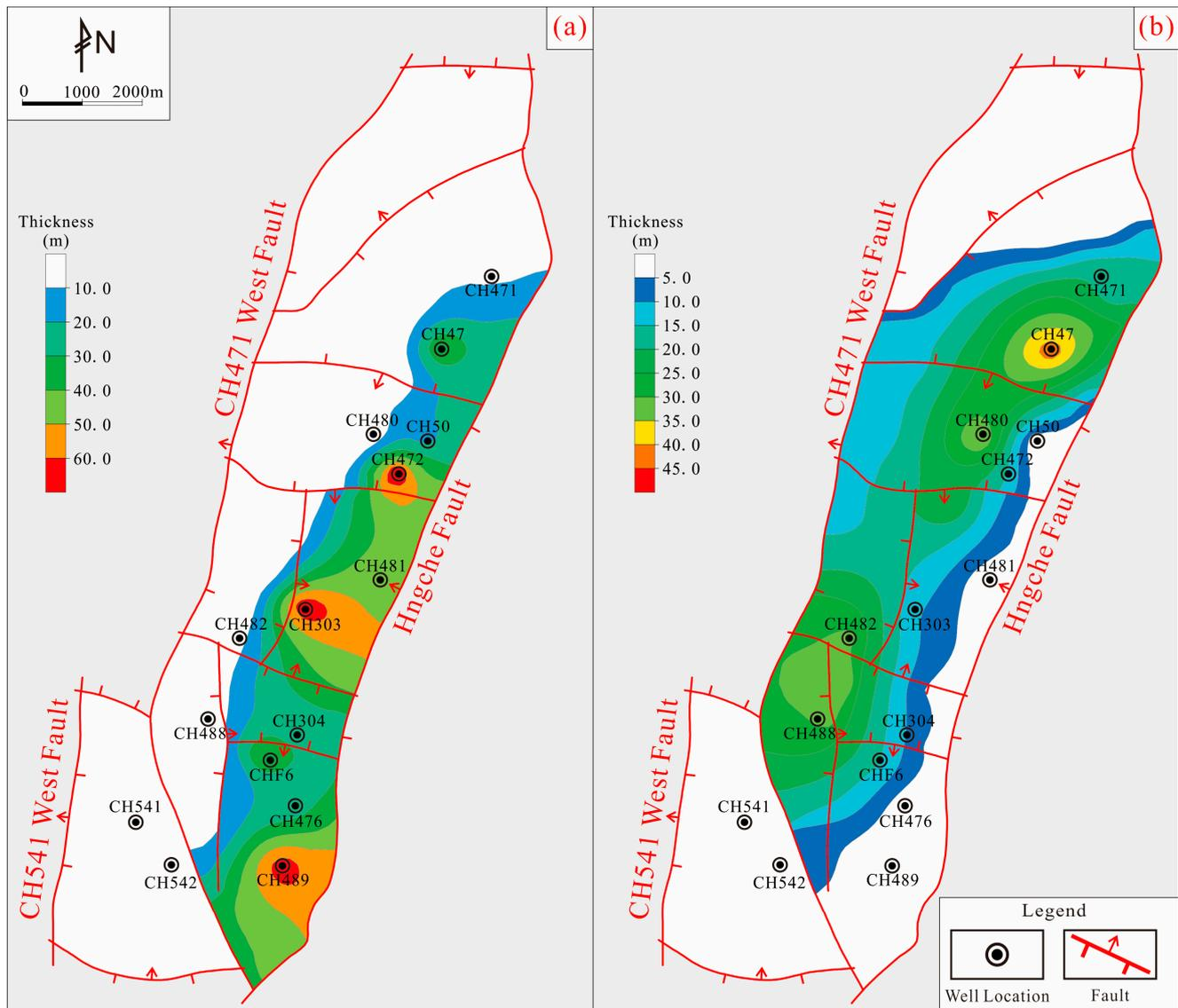
**Figure 7.** The distribution map of reservoir plane thickness in the study area. (a) Plane thickness distribution diagram of explosive facies volcanic breccia reservoir; (b) plane thickness distribution diagram of overflow facies basalt and andesite reservoir.
