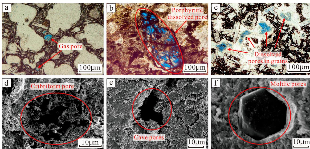
**Figure 4.** Pore types of volcanic reservoirs. (a) Gas pore of basalt, CH541, 2079.05 m. (b) Porphyritic dissolved pore, CH541, 2055.89 m. (c) Dissolved pores in grains, CHF061, 2546.55 m. (d) Cribriform pore, CH541, 2055.89 m. (e) Cave pore, CH542, 2090.86 m. (f) Moldic pore, CH541, 2057.31 m.
