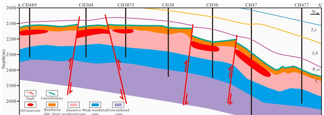
Figure 11. The longitudinal distribution map of weathering degree in the study area.
