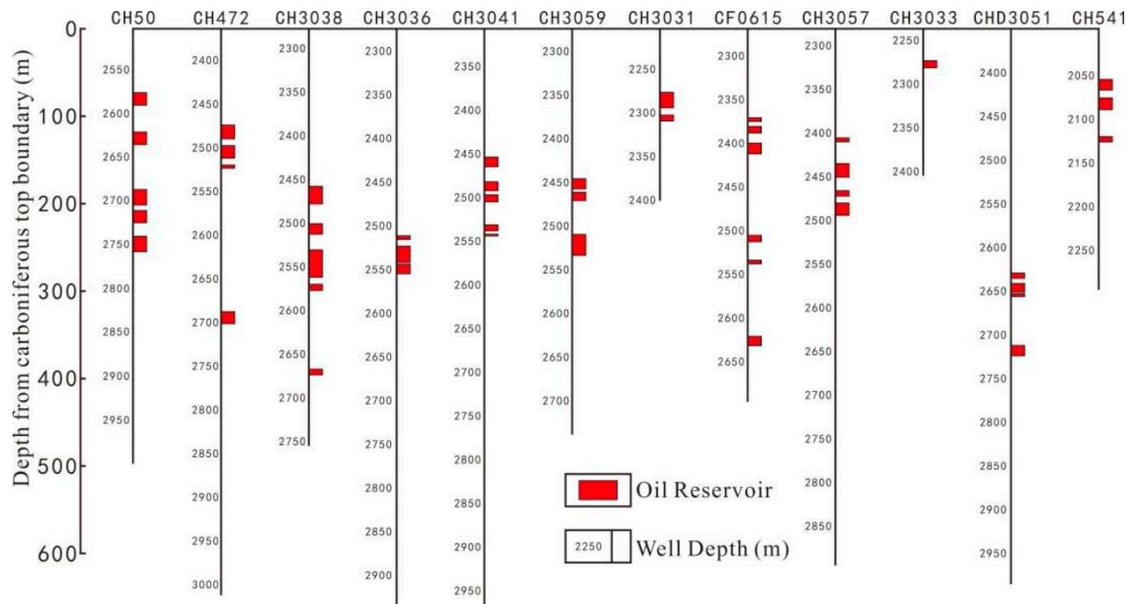
**Figure 12.** The depth of oil-bearing interval from the top boundary of Carboniferous in the study area.
