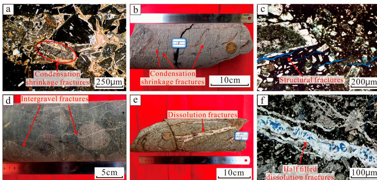
**Figure 5.** Fracture types of volcanic reservoir. (a) Microfracture and condensation shrinkage fractures, CH30, 2287.08 m. (b) Condensation shrinkage fractures and tension fractures, CH471, 2625.09–2625.38 m. (c) Structural fractures, CH472, 2956.78 m. (d) Intergravel fractures, CH48, 3165.22–3165.41 m. (e) Dissolution fractures, CH48, 2726.67–2726.97 m. (f) Half-filled dissolution fractures, CHF6, 2506.11 m.
