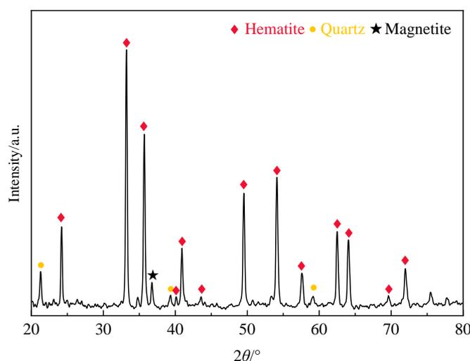
**Figure 1.** XRD analysis of the hematite sample.**Table 2.** Chemical composition analysis of hematite sample.
