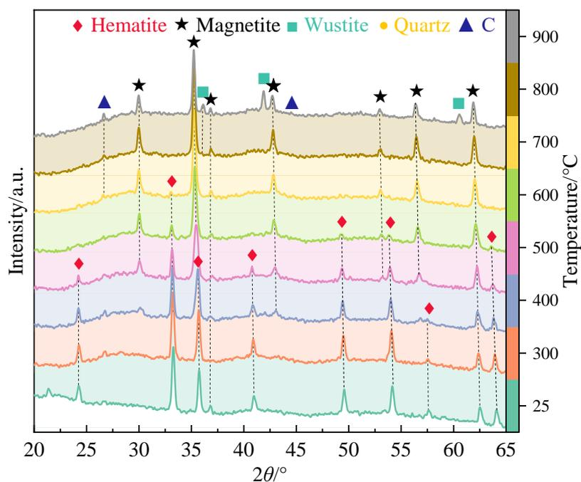
**Figure 5.** In situ heating XRD pattern of corn straw and hematite in N<sub>2</sub> atmosphere (heating rate: 20 °C/min).
