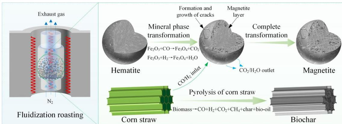
**Figure 7.** Mechanism schematic of corn straw as a green reductant to promote the phase transformation of hematite.
