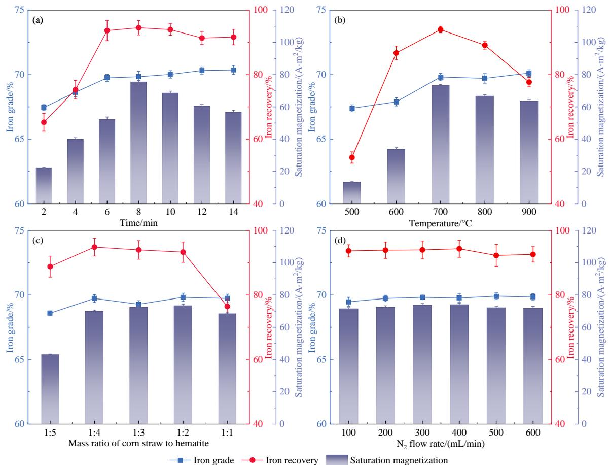
**Figure 3.** Effect of roasting conditions on magnetic separation performance and saturation magnetization, (a) roasting time, (b) roasting temperature, (c) mass ratio of corn straw to hematite, (d)  $N_2$  flow rate.
