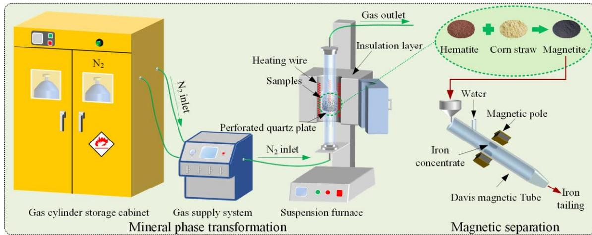
**Figure 2.** Schematic of hematite mineral phase transformation test with corn straw as green reductant.
