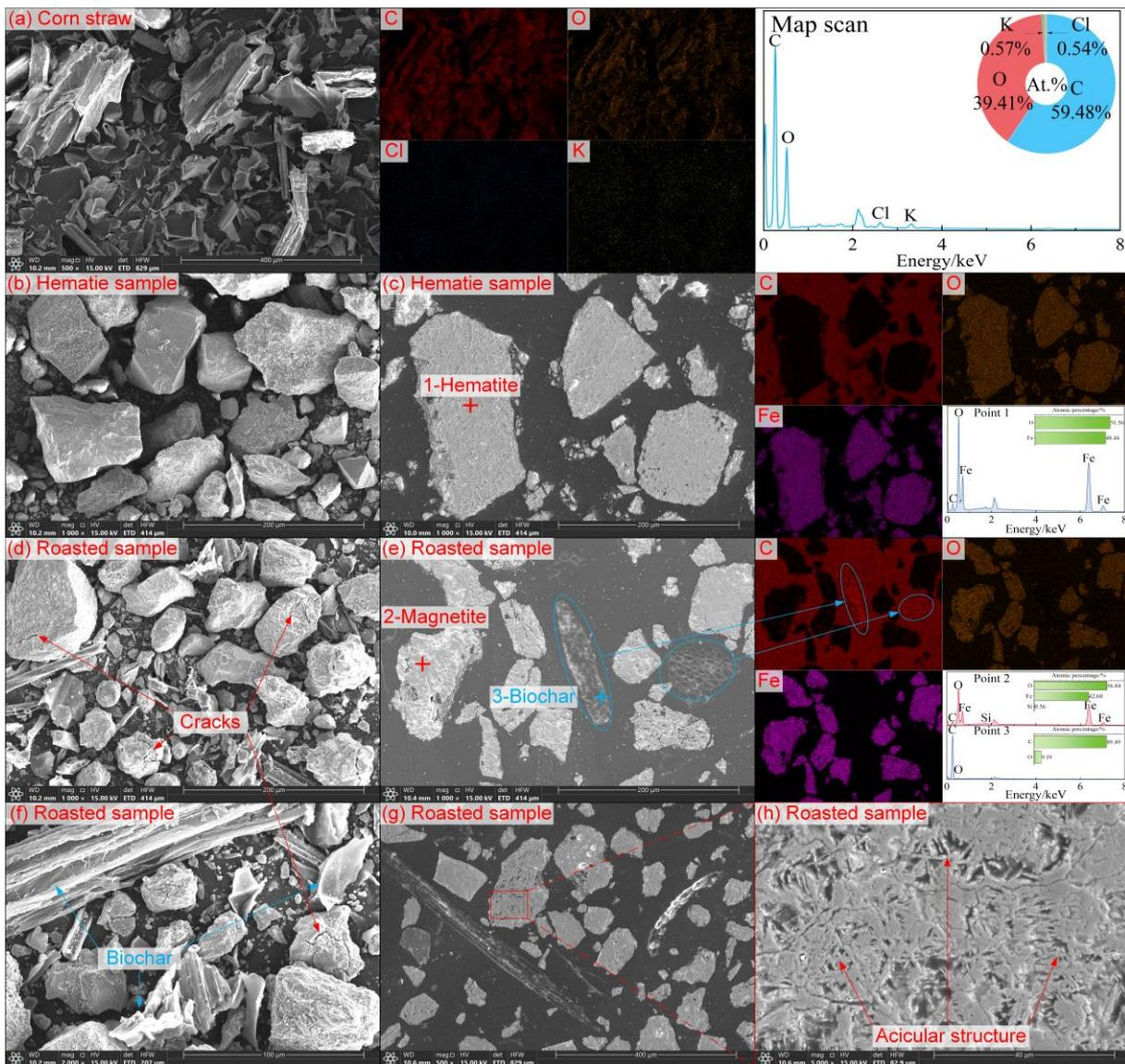
**Figure 6.** Microstructure analysis: (a) SEM image and map scan of corn straw, (b) SEM image of hematite sample particles, (c) SEM image and map scan of cross section of hematite sample, (d,f) SEM images of roasted sample particles, (e) SEM image and map scan of cross section of roasted sample, (g,h) SEM image of roasted sample.
