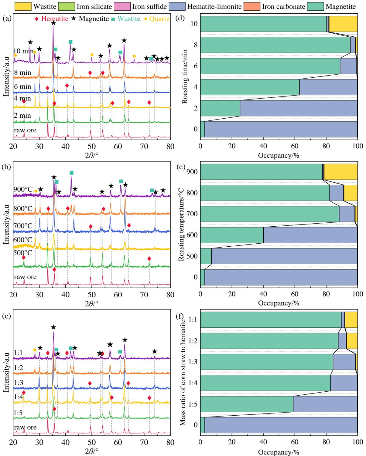
**Figure 4.** XRD pattern and iron phase composition of roasted samples: (a,d) effects of roasting time; (b,e) effects of roasting temperature; (c,f) effects of corn straw dosage.
