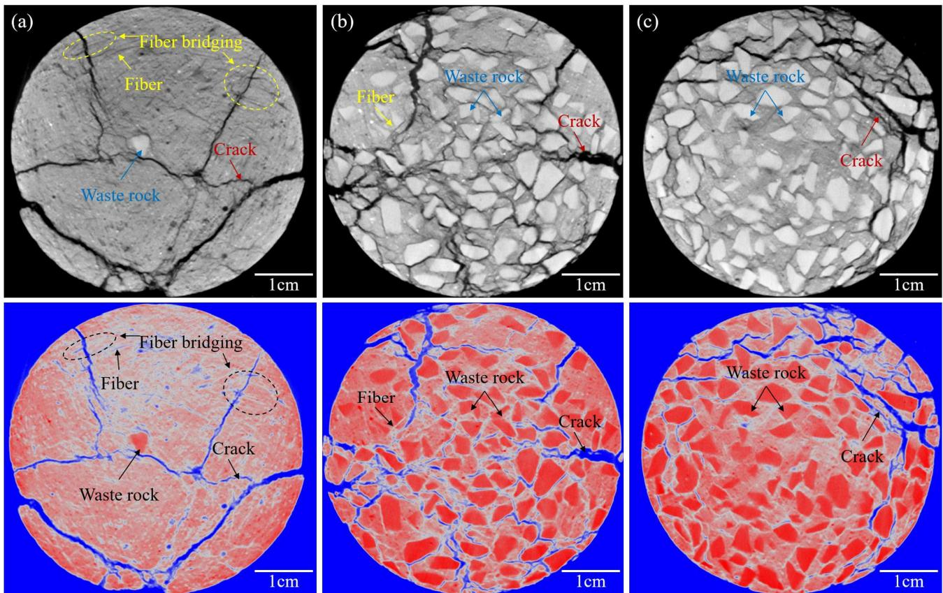
**Figure 5.** 2D CT images of PP6-0.6: (a) Z = 80 mm; (b) Z = 50 mm; (c) Z = 20 mm.
