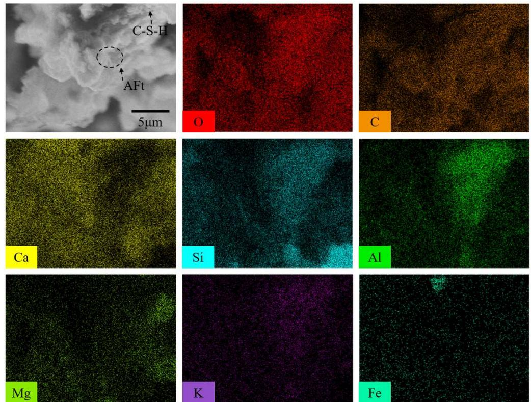
Figure 13. The main element mapping distributions of FRCTWRF sample.
