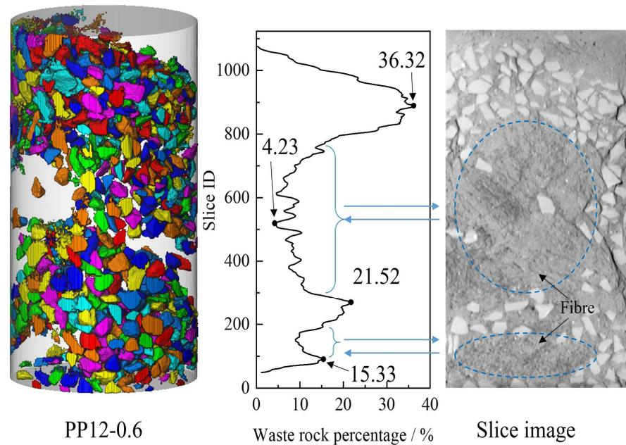
Figure 8. Distribution pattern of waste rock within PP12-0.6.
