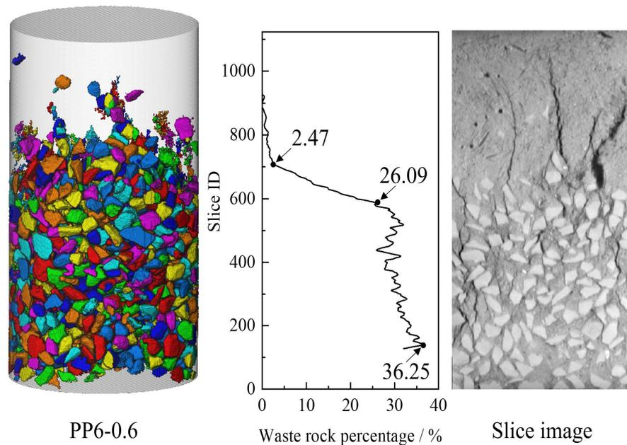
Figure 7. Distribution pattern of waste rock within PP6-0.6.
