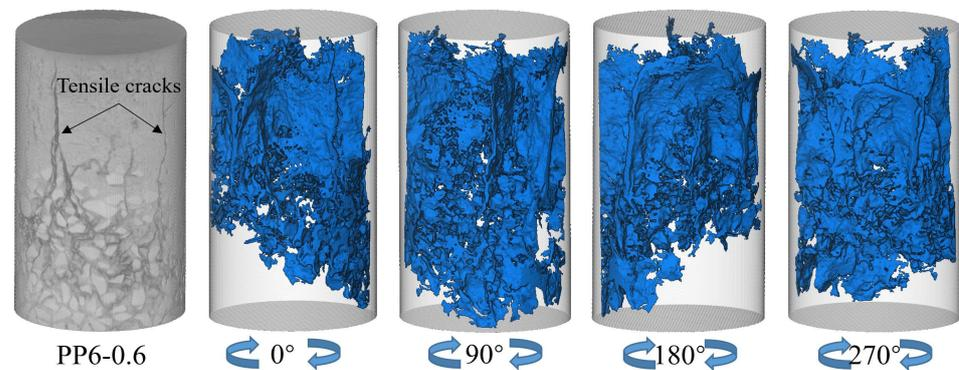
Figure 9. 3D reconstructed image of the cracks in PP6-0.6.
