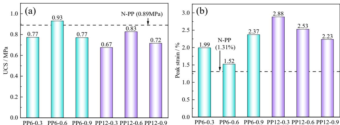
**Figure 3.** UCS and peak strain of FRCTWRF samples: (a) UCS; (b) peak strain. Cyan means PP6; purple means PP12.
