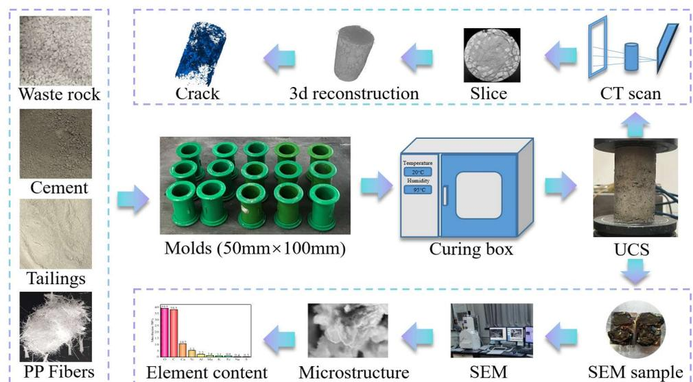
**Figure 2.** A flow chart of specimen preparation processes, including innovative materials/methods.
