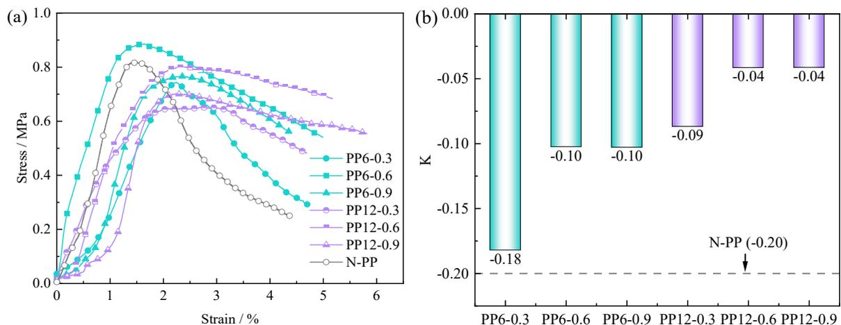
**Figure 4.** Stress–strain curves and slopes of post-peak curves for FRCTWRF specimens: (a) stress–strain plots; (b) slopes of post-peak curves.
