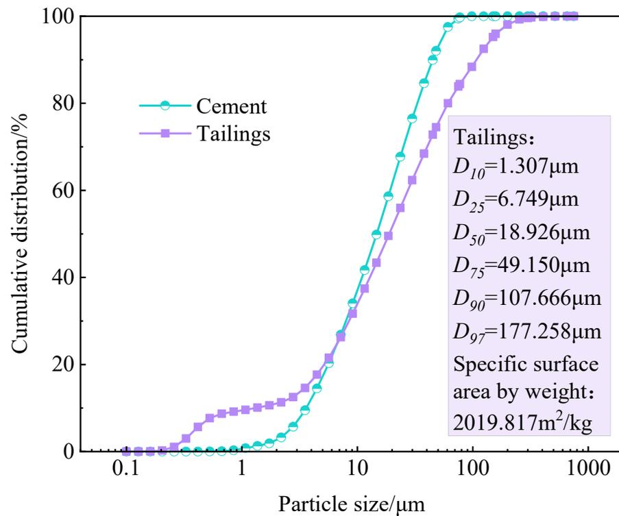
Figure 1. GSD curves for cement and gold tailings.
