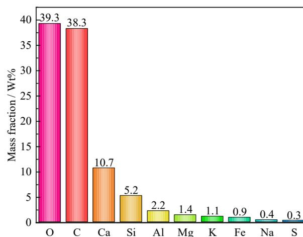
Figure 14. EDS values for hydrated products of FRCTWRF sample.
