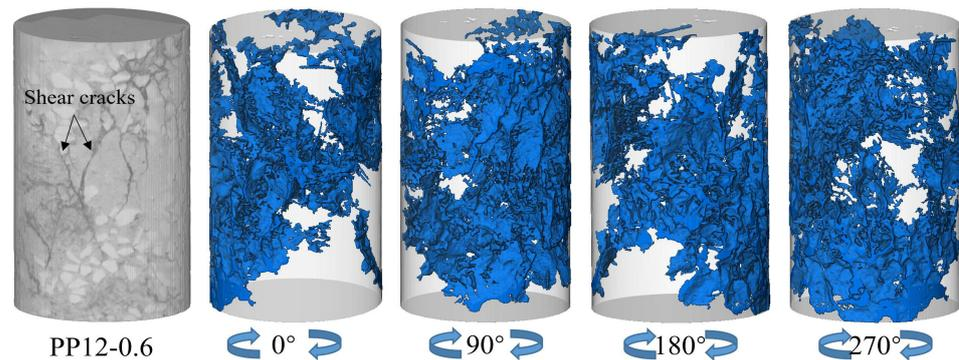
**Figure 10.** 3D reconstructed image of the cracks in PP12-0.6.
