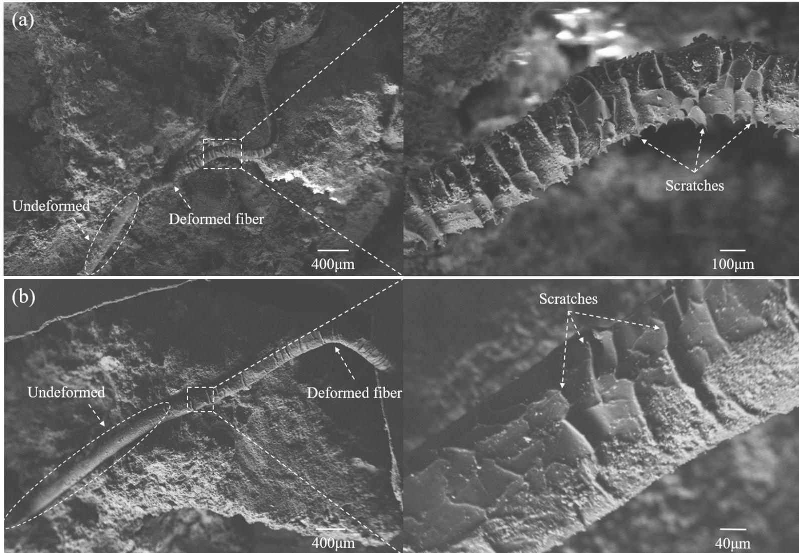
**Figure 12.** Microscopic image of bent and deformed fibers in PP12-0.3. (a) Area 1; (b) Area 2.
