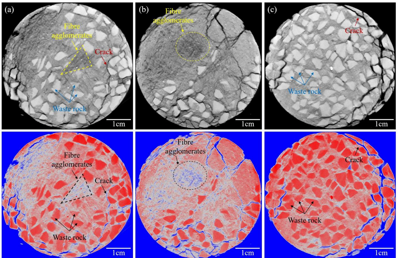
Figure 6. 2D CT images of PP12-0.6: (a) Z = 80 mm; (b) Z = 50 mm; (c) Z = 20 mm.
