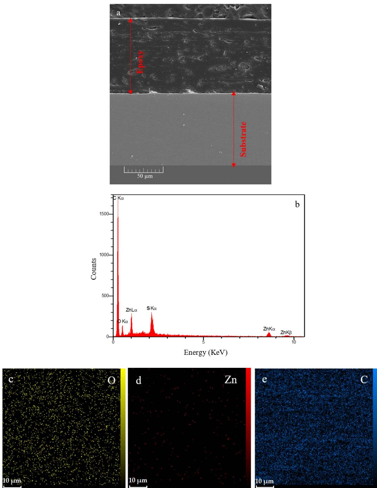
**Figure 8.** Cross-section area of the ZHS-containing nanocomposite (a), together with the corresponding EDS spectrum (b) and elemental maps (c–e).
