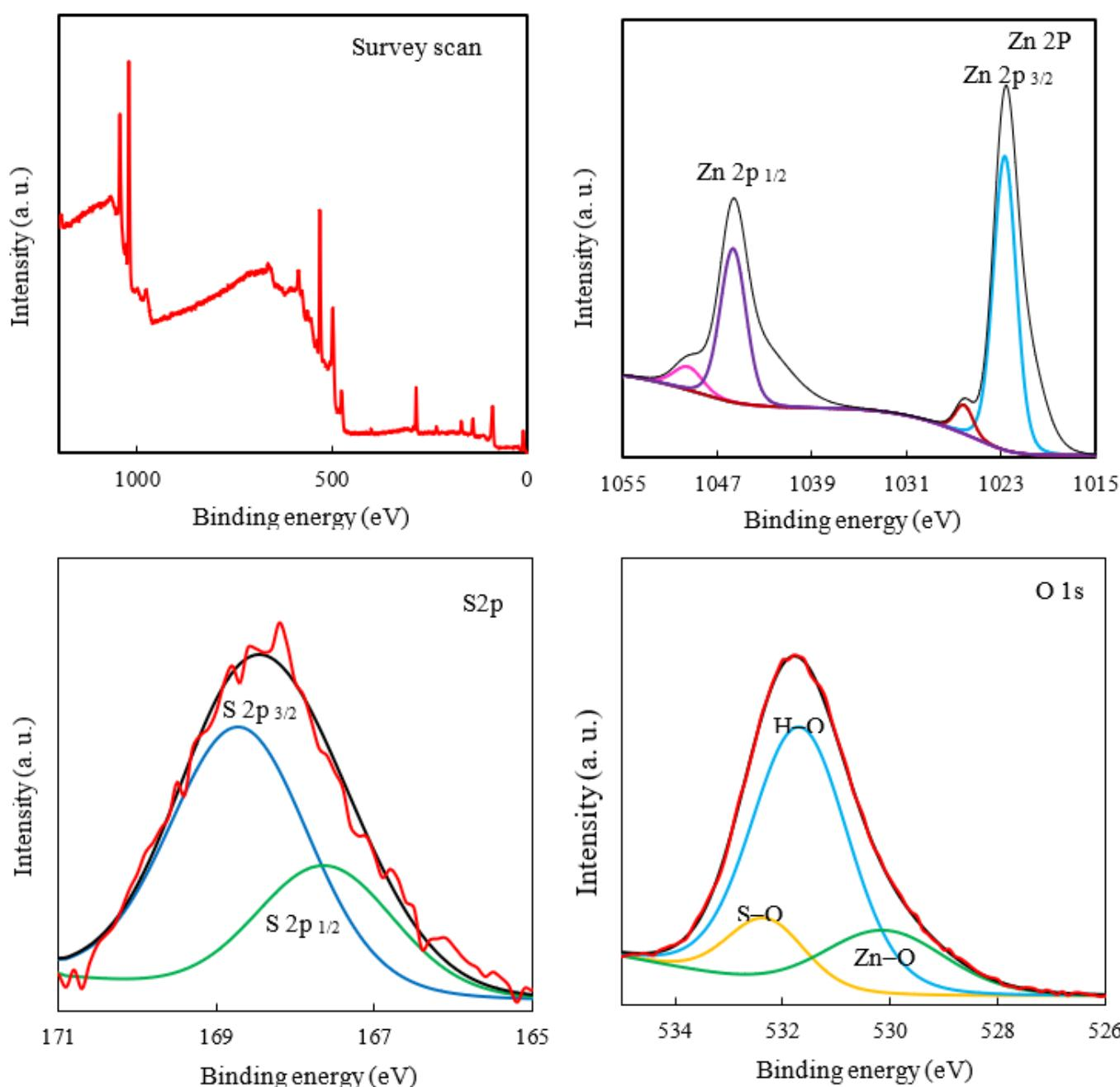
**Figure 3.** The survey scan and high-resolution XPS spectra of the ZHS nanoplates.
