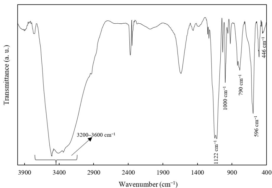
**Figure 2.** The FTIR spectrum of the as-synthesized ZHS nanoplates.
