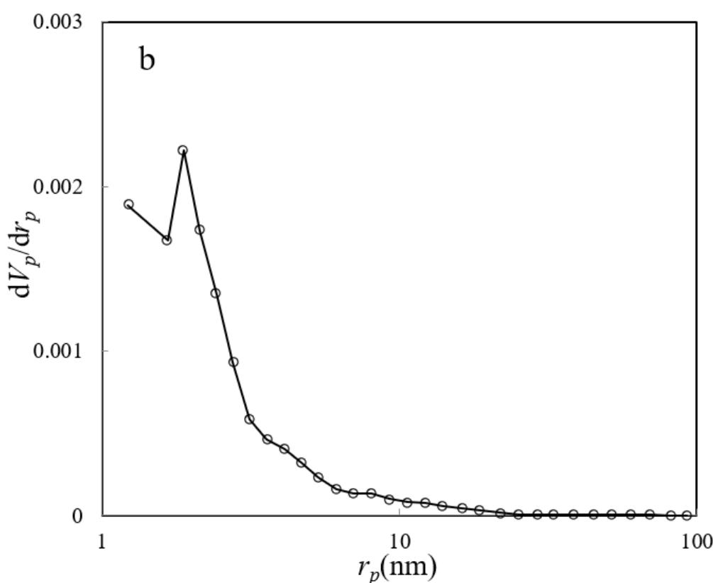
**Figure 5.** BET nitrogen adsorption–desorption (a) and BJH plot (b) of the ZHS nanoplates.
