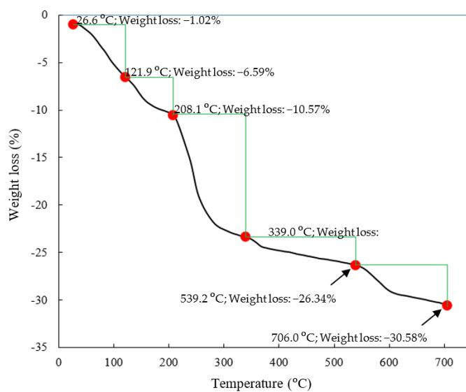
**Figure 4.** TGA curve of the synthesized ZHS nanoplates.
