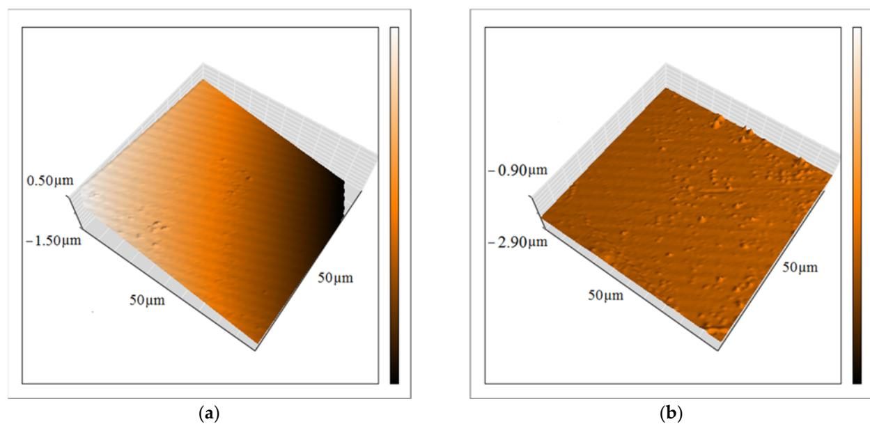
**Figure 9.** Topography of the neat (a) and ZHS-containing (b) epoxy coatings obtained by the AFM.
