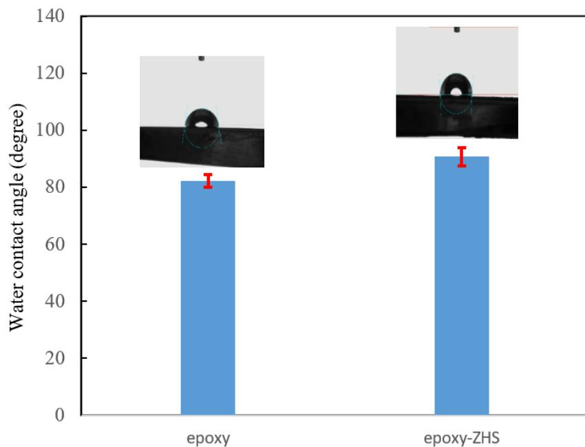
**Figure 10.** Water contact angle of the neat and ZHS-containing epoxy coatings.
