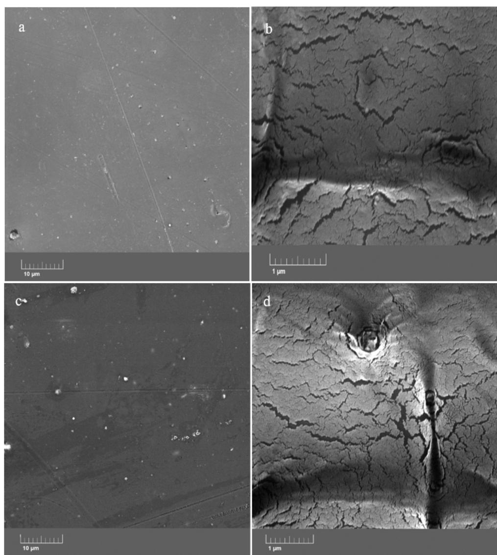
**Figure 6.** FESEM images of the neat (**a,b**) and ZHS-containing (**c,d**) epoxy coatings.
