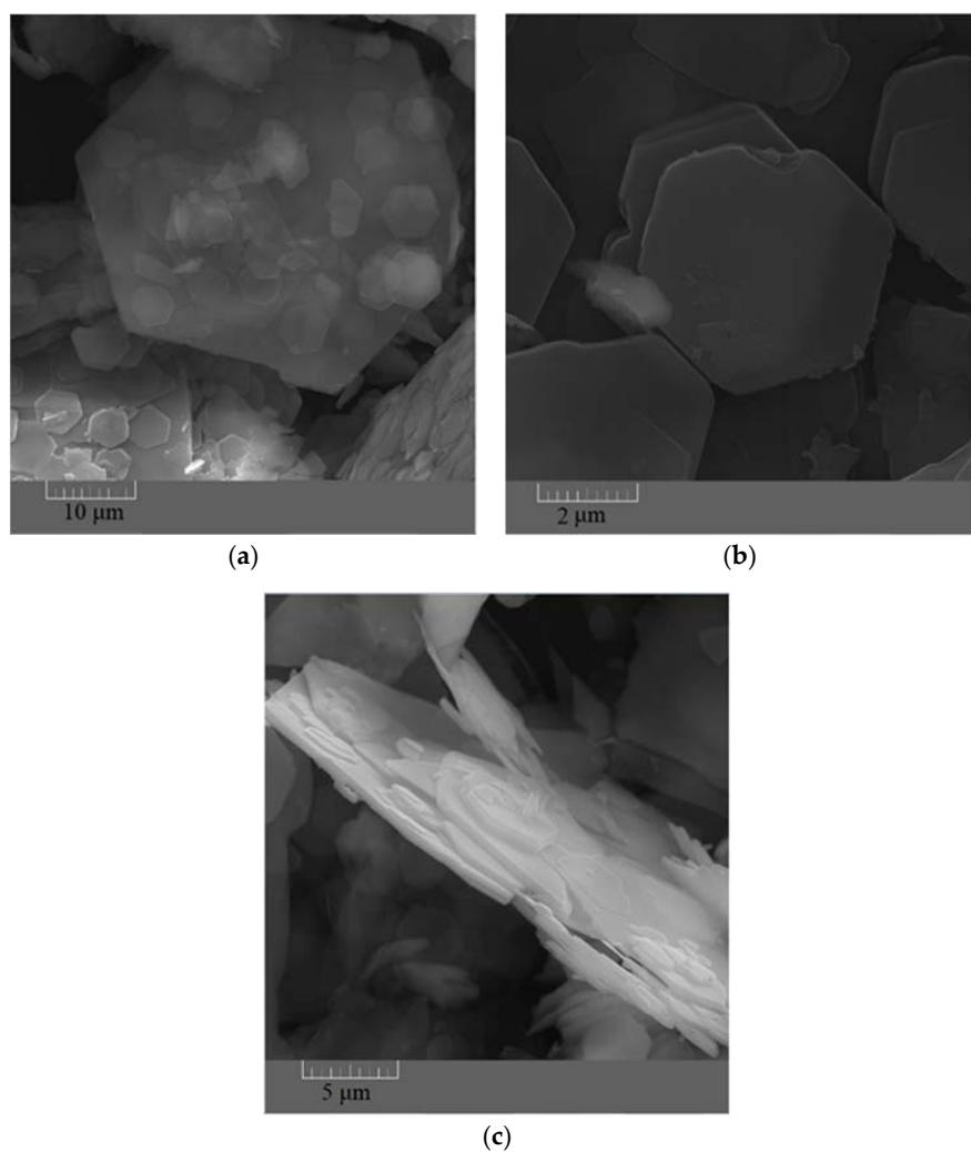
**Figure 1.** FESEM images showing shape (a,b) and thickness (c) of the synthesized ZHS nanoplates.
