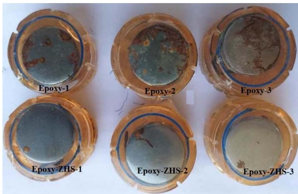
**Figure 12.** The visual images of the neat and ZHS-containing epoxy coatings after the corrosion tests.
