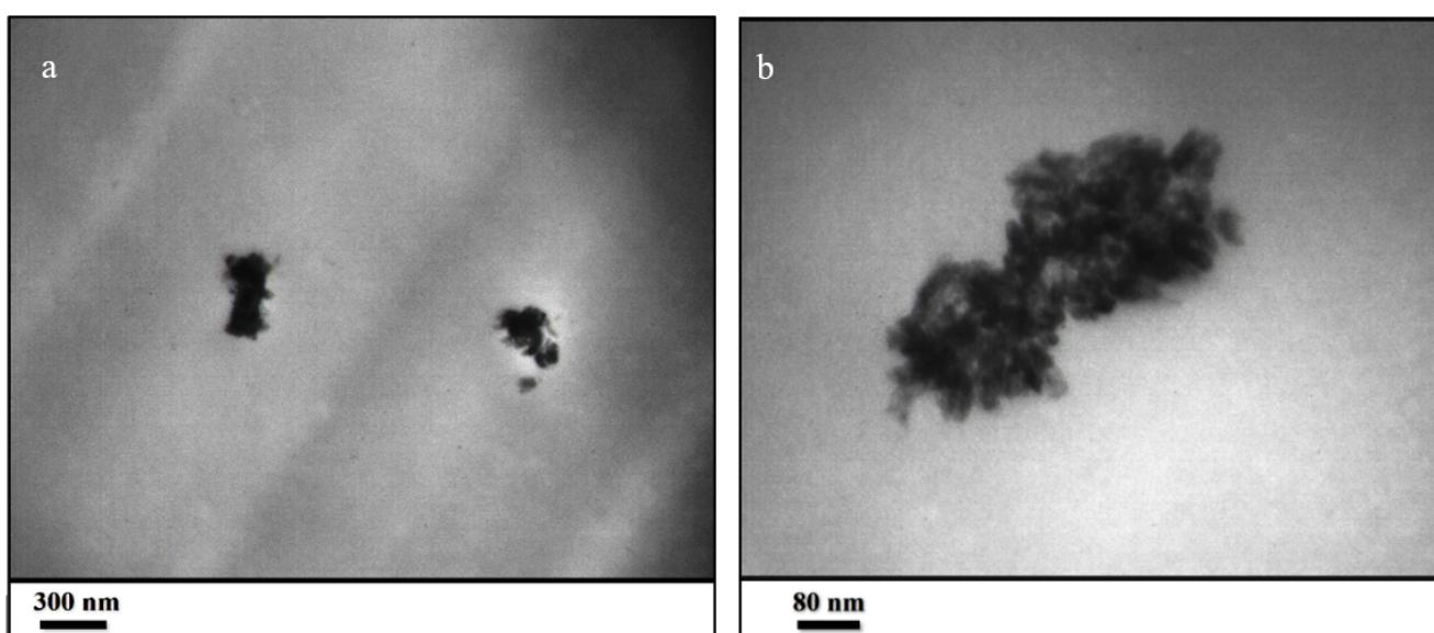
**Figure 7.** TEM images at low (a) and high (b) magnifications taken from the thin slice of the ZHS-containing epoxy resin prepared by the ultramicrotomy.
