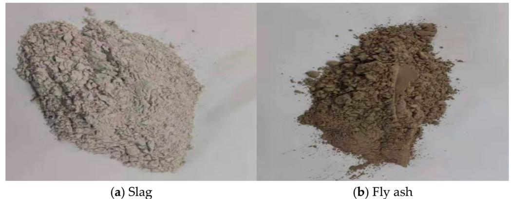
**Figure 2.** Slag and fly ash samples.
