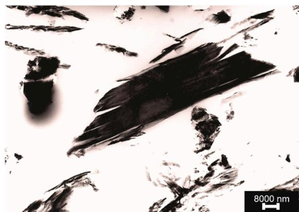
**Figure 4.** TEM micrograph of finely ground talc (<20  $\mu\text{m}$ ) embedded in a resin and cut perpendicularly to the basal plane of particles.
