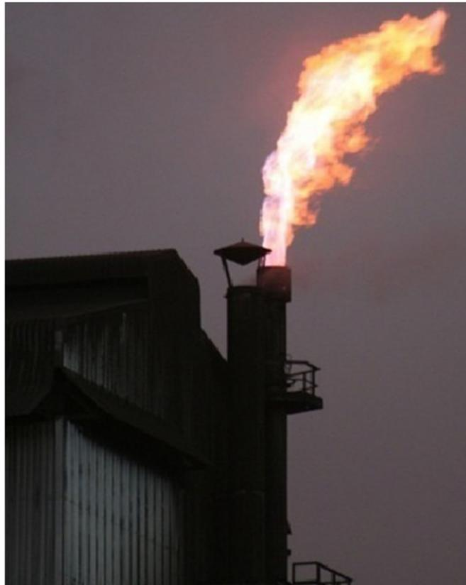
**Figure 13.** A typical off-gas flare on top of a closed SAF stack [107,108]. Reproduced from Reference [107] with permission from Springer under Creative Commons Attribution 4.0 International License <http://creativecommons.org/licenses/by/4.0/> (accessed on 2 May 2023).
