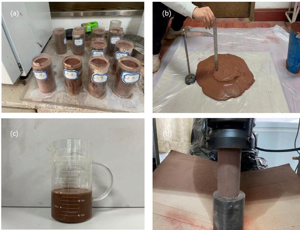
**Figure 3.** (a) Preparation of specimen; (b) Slump test; (c) Bleeding rate test; (d) Unconfined compression test.
