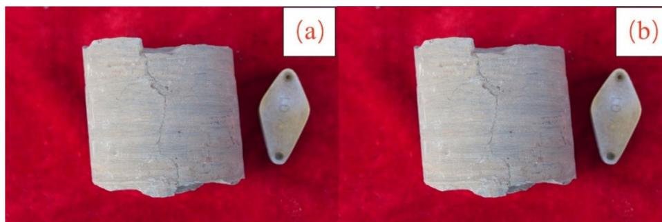
**Figure 20.** Characteristics of the sandstone core fractures in the Zhiluo Formation: (a) fractures and (b) detachment.
