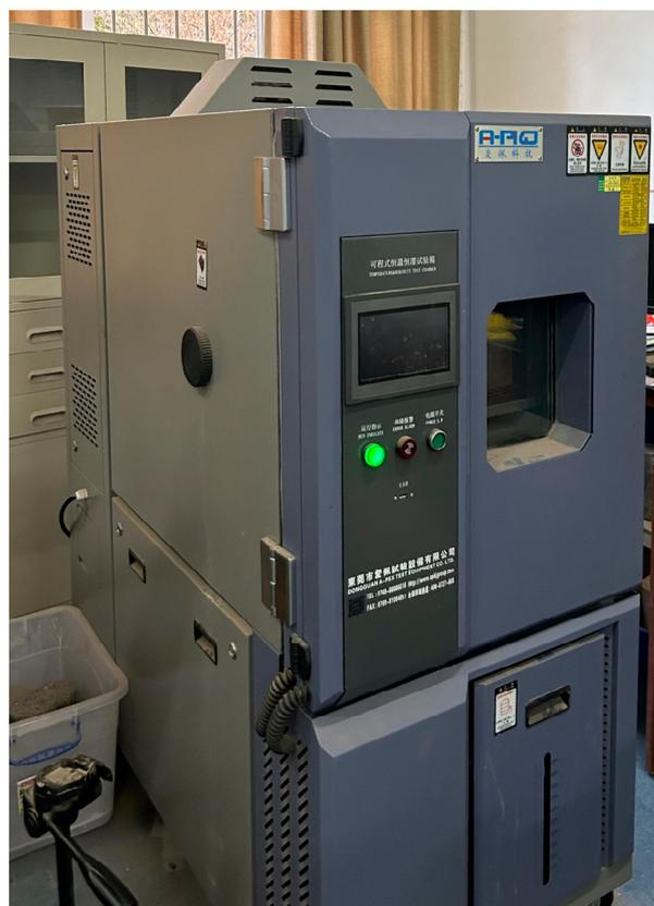
(b) Temperature Shrinkage Test
