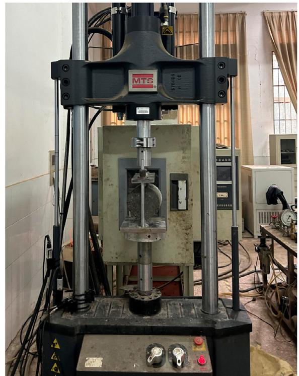
(b) Splitting strength test
