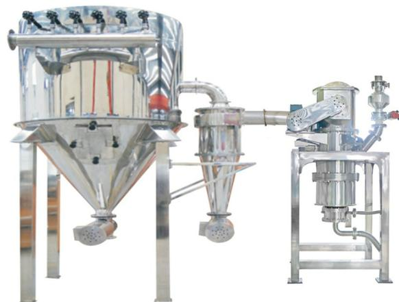
**Figure 13.** Experimental fluidized bed opposed jet mill.
