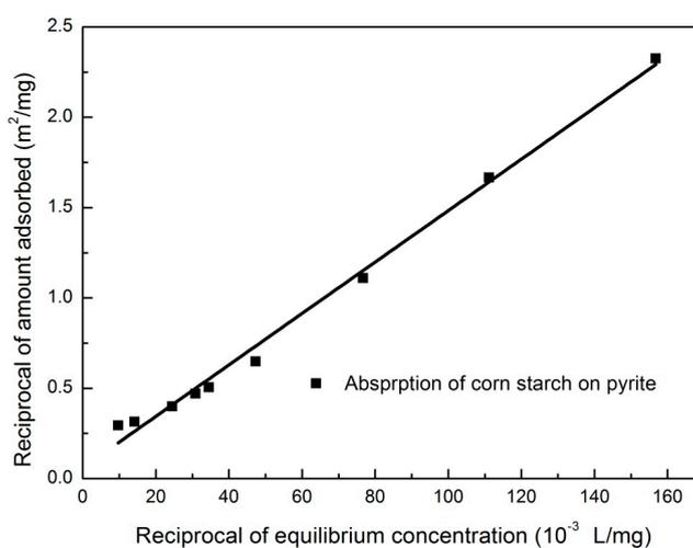
Figure 9. Plot of the reciprocal of adsorption density versus reciprocal of equilibrium concentration.
