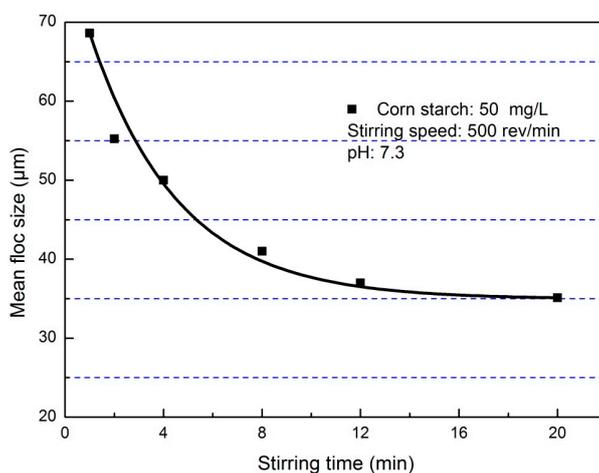
Figure 4. Effect of the stirring time on the size of pyrite flocs with corn starch.
