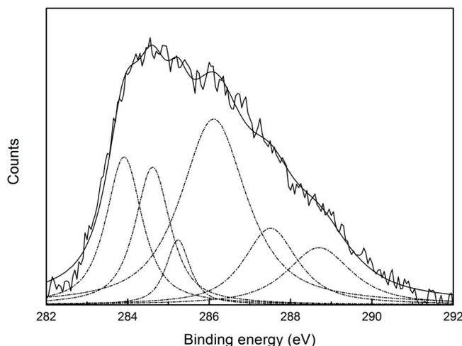
Figure 12. C 1s spectrum of corn starch after adsorption on the pyrite surface.
