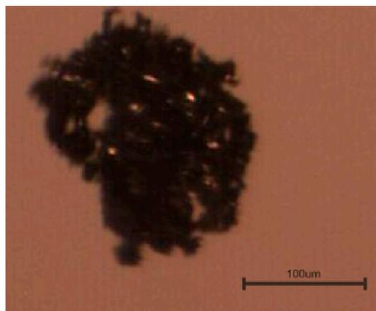
**Figure 6.** Optical microscopy image of pyrite flocs in the presence of corn starch.
