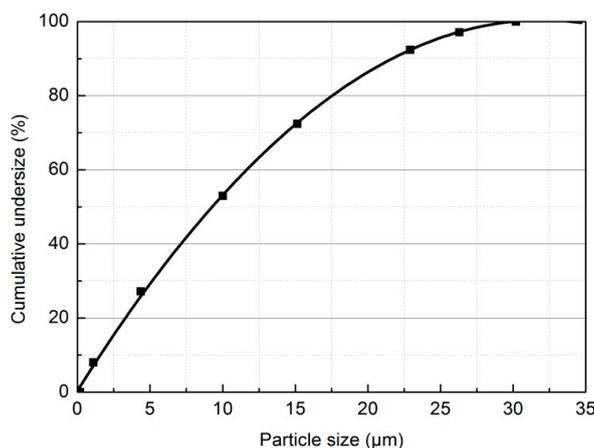
Figure 1. Size distribution of pyrite fines.
