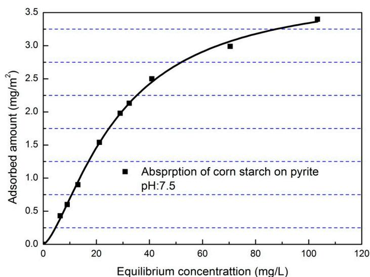
Figure 8. Adsorption isotherm of corn starch onto pyrite.
