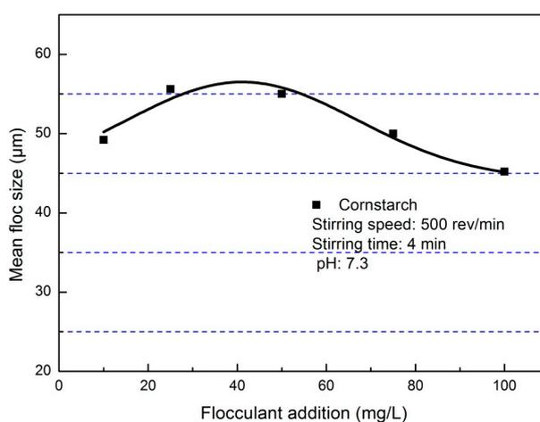
Figure 5. Effect of the flocculant addition on the size of pyrite flocs with corn starch.
