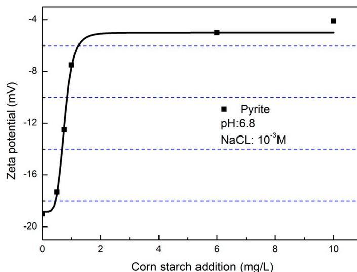
Figure 11. Effect of the corn starch addition on the zeta potential of pyrite.
