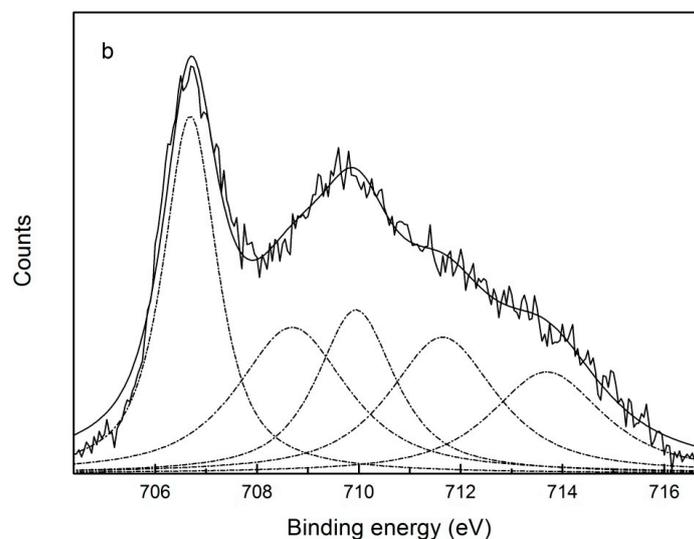
**Figure 13.** Fe 2p<sub>3/2</sub> spectra of pyrite before (a) and after (b) the adsorption of corn starch.
