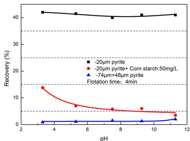
**Figure 7.** Effect of pH on the recovery of pyrite fines in froth flotation with and without the flocculant.
