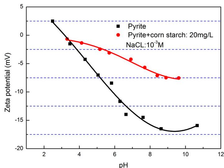
Figure 10. Zeta potential of pyrite as a function of pH without and with corn starch.
