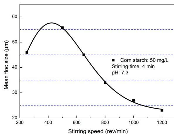
Figure 3. Effect of the stirring speed on the size of pyrite flocs with corn starch.
