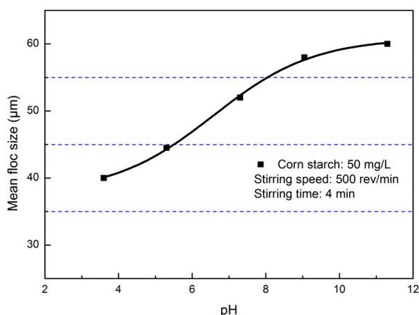
Figure 2. Effect of pH on the mean size of pyrite flocs in the presence of corn starch.
