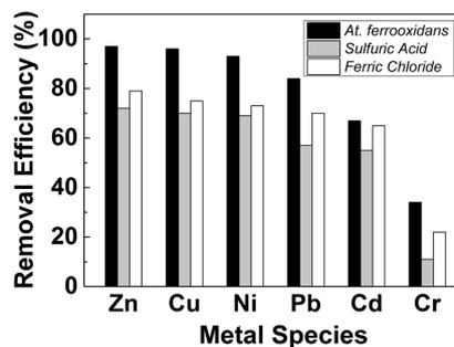
**Figure 1.** Metal removal efficiencies obtained by chemical (i.e., sulfuric or ferric chloride leaching) and bioleaching using *A. ferrooxidans*. The results were obtained at optimum operating conditions: pH, 2; pulp density, 2% (*w/v*); agitation speed, 120 rpm; and, temperature,  $25 \pm 2$  °C. Data obtained from Bayat and Sari 2010 [22].
