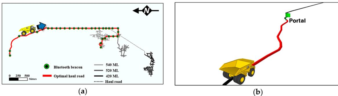
**Figure 8.** Screenshots of BBUNS application when the signal of a Bluetooth beacon with minor ID 3 is recognized. (a) Two-dimensional view of the optimal haul road showing the current location of the dump truck, the travel direction, and Bluetooth beacons installed along the path; (b) Three-dimensional view of the optimal haul road.
