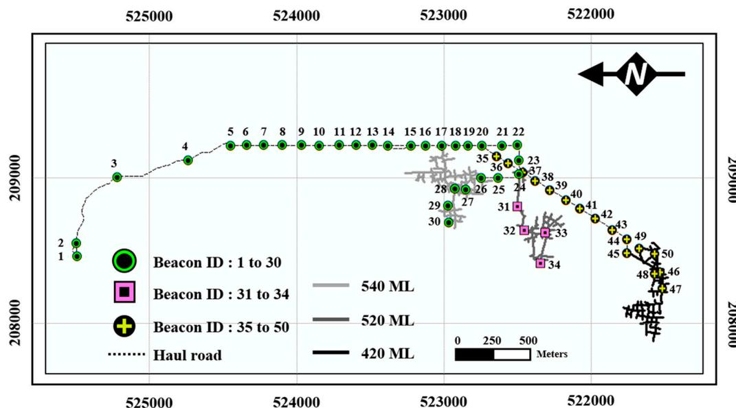
Figure 5. Underground mine map showing the installation position of Bluetooth beacons.
