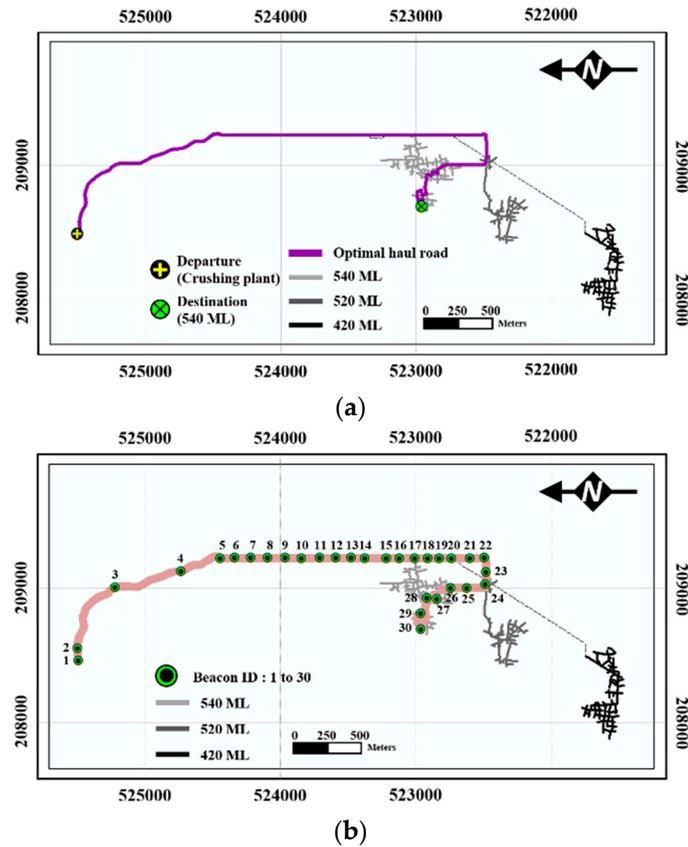
**Figure 7.** (a) Optimal haul road connecting the crushing plant and 540 ML workplace; (b) Bluetooth beacons that installed along the optimal haul road.
