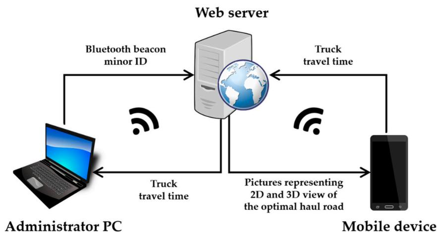
**Figure 6.** Conceptual view of data exchanges that occur when Bluetooth beacon-based underground navigation system (BBUNS) recognizes the signal of Bluetooth beacon that has minor ID 1.
