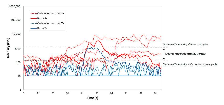
**Figure 6.** Se and Te LA-ICP-MS trace element line transects for Brora coal pyrite and Carboniferous coals pyrite samples, showing Brora Te peak intensity an order of magnitude higher than Carboniferous coals.
