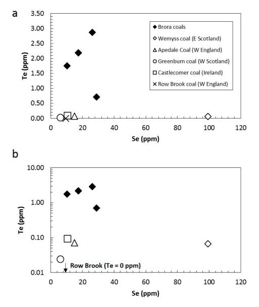
**Figure 5.** LA-ICP-MS Te vs. Se in pyrite cross-plot showing Brora coal-hosted pyrite compared to other pyrite hosted in British and Irish Carboniferous coals: (**a**) normal scale; and (**b**) log scale.
