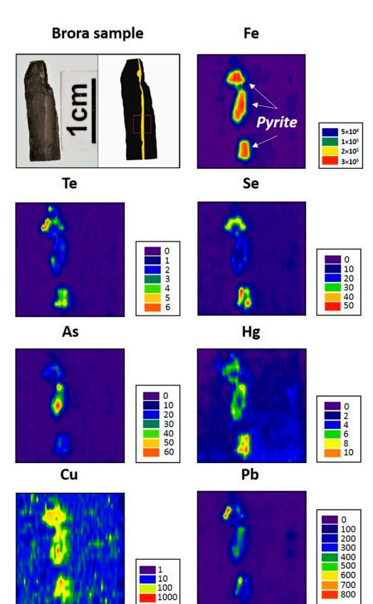
**Figure 2.** Brora coal, digitised sample and laser ablation inductively coupled plasma-mass spectrometry (LA-ICP-MS) trace element maps. Map size 25 mm  $\times$  25 mm.
