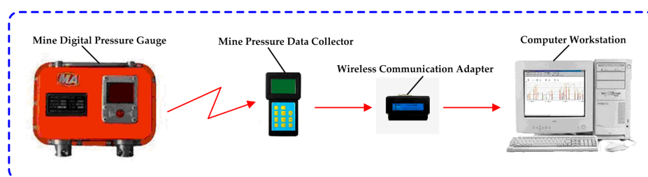
Figure 9. Schematic of the pressure recording system.
