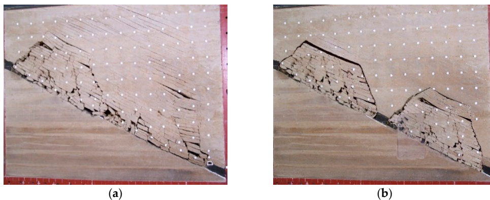
Figure 17. Excavation of 1411 panels in physical models. (a) LMSG; (b) CLTCC.
