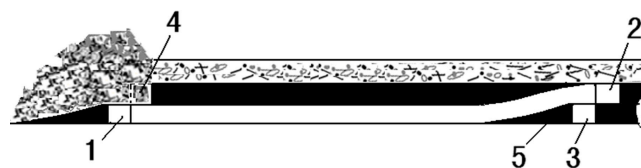
Figure 3. Typical LMSG (Longwall Mining with Split-level Gate roads) top coal caving mining layout in relatively flat coal seams (Figure prepared courtesy of Zhao [13]). 1—Tail gate of the active panel (Panel 1); 2—Head gate of the active panel (Panel 1); 3—Tail gate of the successive panel (Panel 2); 4—Head gate of the previous panel (Panel 1); 5—Triangular x -section coal pillar loss.
