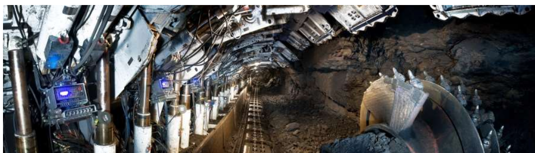
Figure 1. Typical VMM longwall face equipment.
