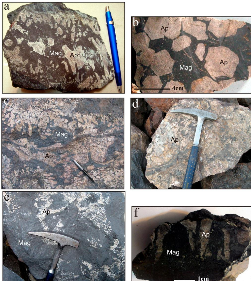
**Figure 3.** Photographs of representative samples from the main apatite-magnetite associations in Chadormalu. (a,b) Magnetite-apatite association from veins in the altered host rocks. (c) Apatite grains and grain aggregates in the marginal part of the main ore body. (d) Brecciated apatite and associated magnetite in the marginal parts of the main ore body. (e,f) Irregular apatite veinlets and streaks in the main ore body. Abbreviations: Ap = apatite; Mag = magnetite.
