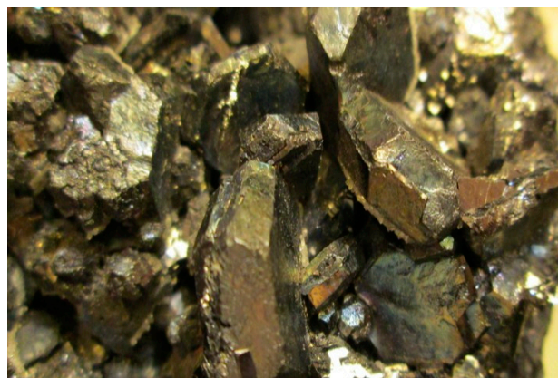
Figure 6. Photograph showing six or seven 1 cm platy galena crystals indicating that they not only consist of two twin portions but also show that the twins are penetration twins.
