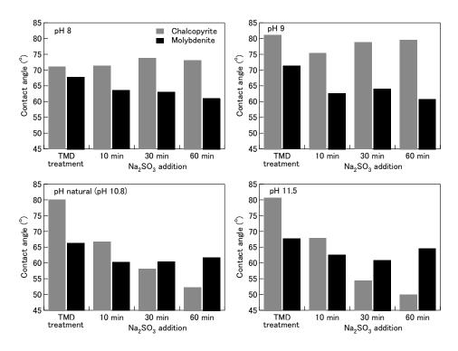
**Figure 1.** Contact angle of chalcopyrite and molybdenite at various pH values after the pretreatment using TMD solution followed by treatment using 0.1 M Na<sub>2</sub>SO<sub>3</sub> for 10–60 min.
