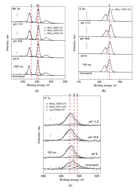
**Figure 4.** The Mo3d (**a**); S2p (**b**); and O1s (**c**) spectra of untreated and treated molybdenite with 0.1 M Na<sub>2</sub>SO<sub>3</sub> treatment at various pH conditions.
