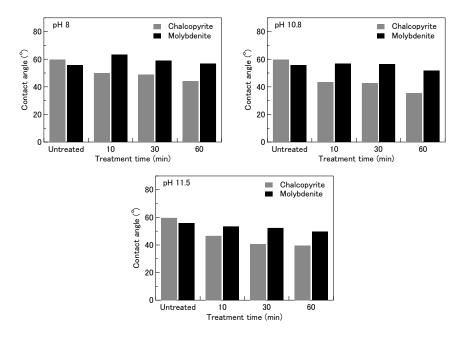
**Figure 2.** Effect of 0.1 M Na<sub>2</sub>SO<sub>3</sub> on contact angle of chalcopyrite and molybdenite at various pH values and treatment times without pretreatment using TMD solution.
