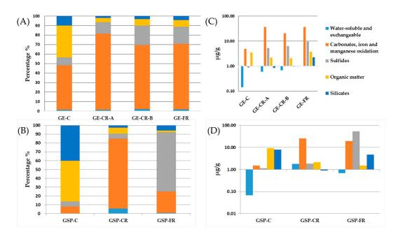
**Figure 16.** Sequential chemical leaching results for nickel: (**A**,**B**) percentage leached; and (**C**,**D**) the concentration in leachates.
