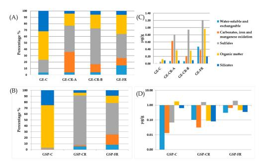
**Figure 7.** Sequential chemical leaching results for molybdenum: **(A,B)** percentage leached; and **(C,D)** the concentration in leachates.
