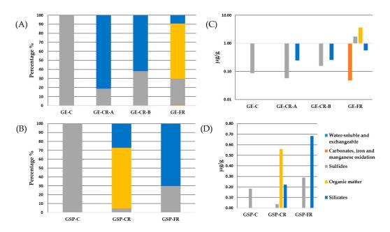
**Figure 13.** Sequential chemical leaching results for selenium: (**A**,**B**) percentage leached; and (**C**,**D**) the concentration in leachates.
