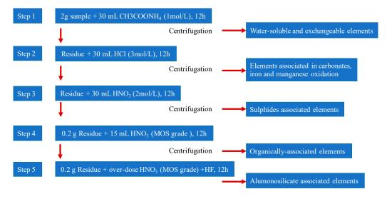
Figure 1. Diagram of the sequential chemical extraction method.
