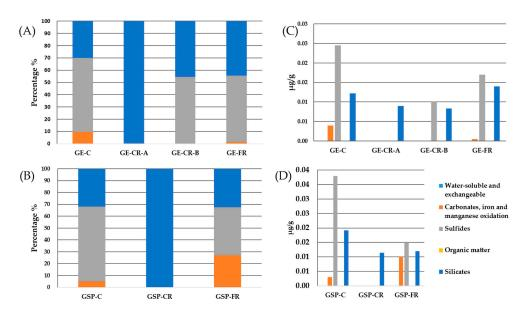
**Figure 6.** Sequential chemical leaching results for mercury:(**A**,**B**) percentage leached; and (**C**,**D**) the concentration in leachates.
