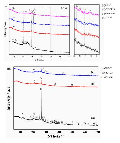
**Figure 2.** XRD diffractograms of minerals in the feed coal and gasification residues: (**A**) samples from the coal to methanol plant (GE); and (**B**) samples from the coal to olefin plant (GSP). K-kaolinite; Q-quartz; Ca-calcite; Ge-gehlenite; S-siderite; P-pyrite; Me-melilite; PF-potassium feldspar; and Pl-plagioclase.
