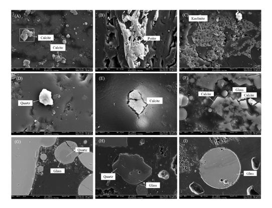
**Figure 3.** Minerals and glass in the gasification residues: (**A**) calcite in GE-C; (**B**) pyrite in GSP-C; (**C**) kaolinite in GSP-C; (**D**) quartz in GSP-C; (**E**) calcite in GSP-CR; (**F**) calcite and glass in GSP-FR; (**G**) quartz and glass in GE-CR (SEM, (**A**–**F**) secondary electron images; and (**G**–**I**) back-scatting images).
