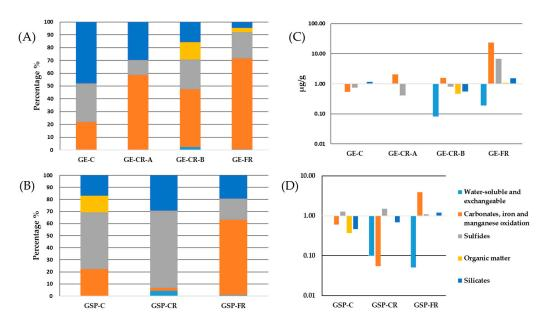
**Figure 12.** Sequential chemical leaching results for arsenic: (**A**,**B**) percentage leached; and (**C**,**D**) the concentration in leachates.
