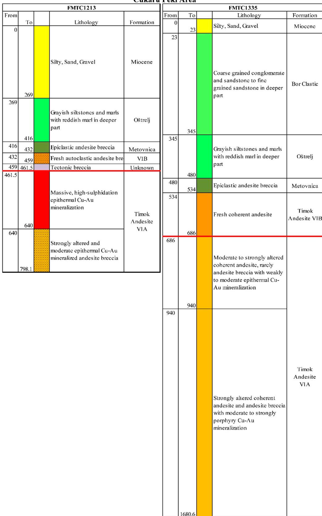
Figure 4. Stratigraphic logs of two drill holes from the Čukaru Peki area (News Release Reservoir Minerals [21,49]). The hatched pattern indicates andesite breccia, whereas the red line marks the boundary between the two andesite subgroups.
