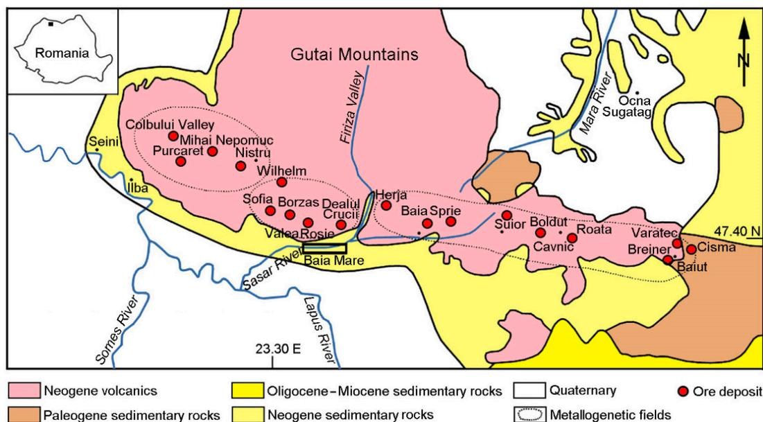
**Figure 2.** Simplified geology of the Baia Mare ore district, NW Romania with location of main ore deposits including Herja (modified after [4]).
