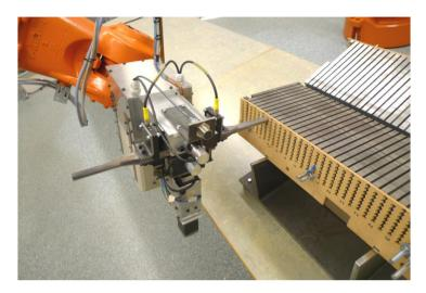
Figure 10 shows the positions of the calibrated WOCS origins for the 400 stator section positional calibrations, relative to the mean value of these measurements. In Figure 11, the corresponding calculated positions of  $\varepsilon$  in the calibrated WOCS are shown. The distance from  $\varepsilon$  to the WOCS origin is set to 1,000 mm in the negative y-direction and 100 mm in the negative z-direction.
