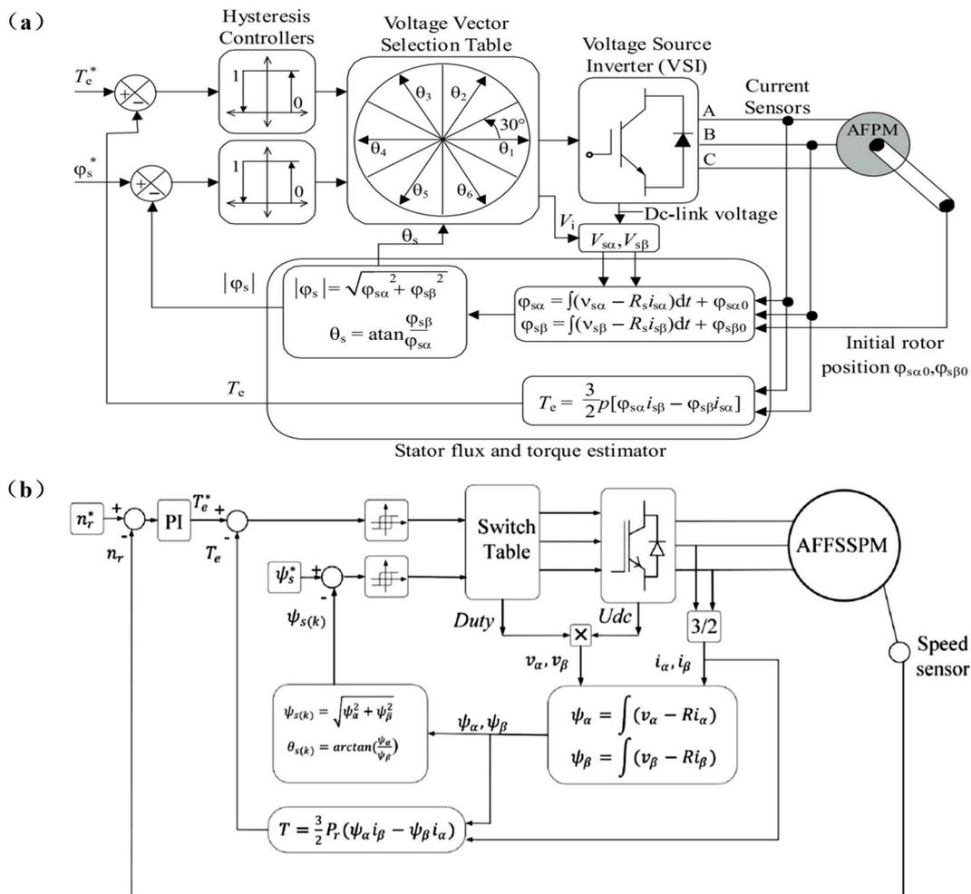
Figure 10. DTC algorithms. (a) DTC algorithm adapted from Ref. [106]. (b) DTFC algorithm adapted with permission from Ref. [107]. Copyright 2017 Emerald Publishing Limited.
