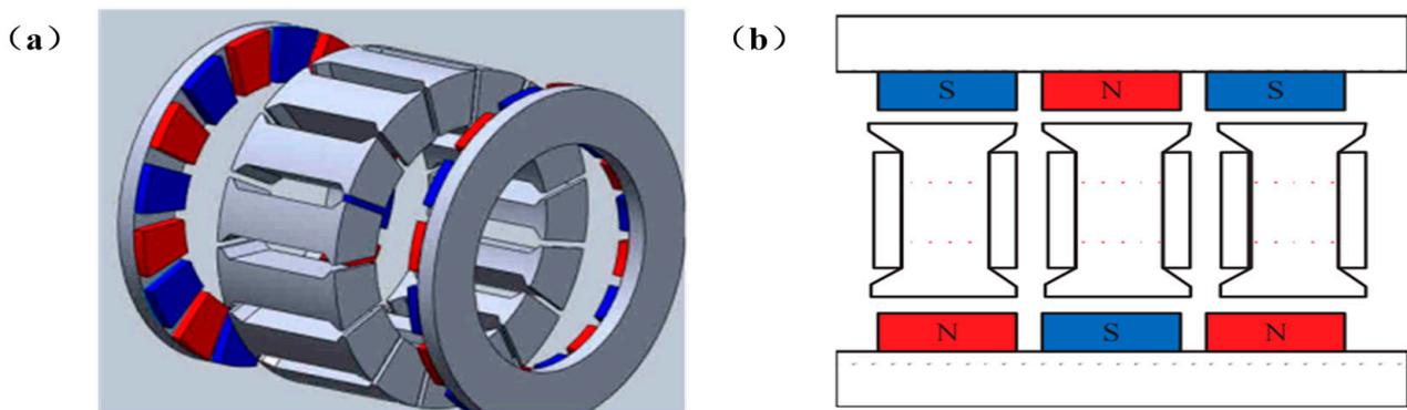
**Figure 5.** The YASA-type AFPM motors: (a) exploded view. Adapted with permission from Ref. [38]. Copyright 2018 John Wiley and Sons. (b) Profile view. Adapted from Ref. [31]. Copyright 2018 MDPI.
