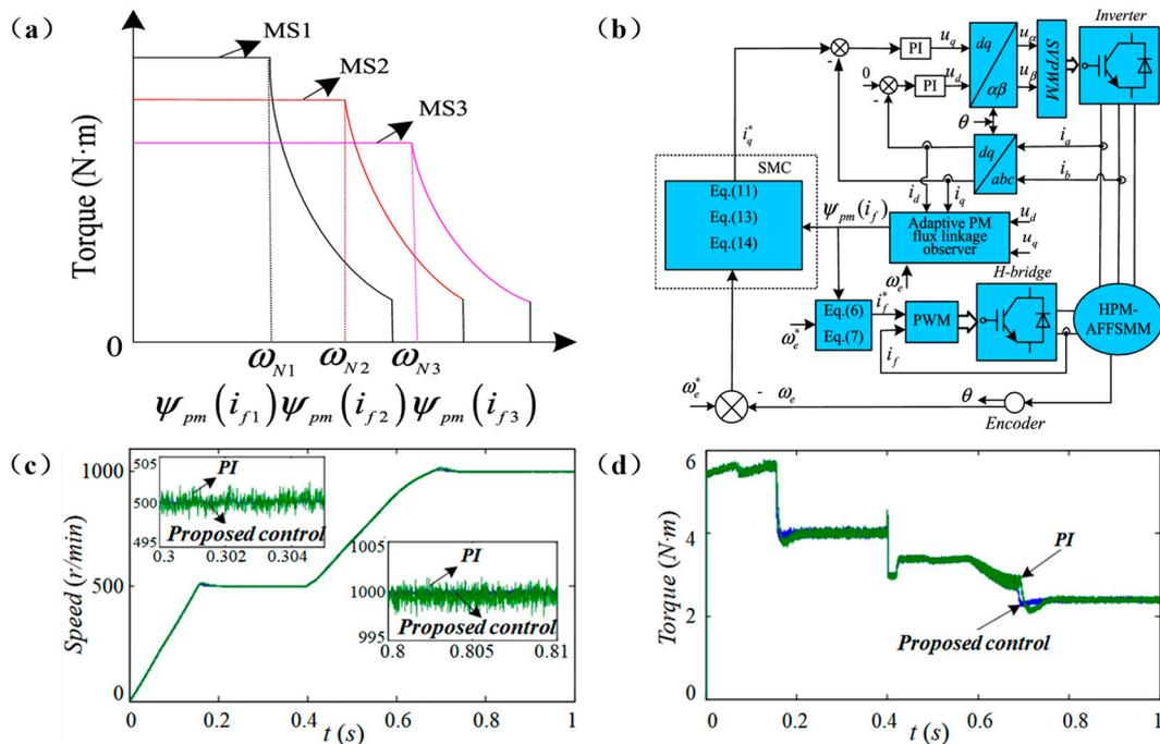
**Figure 11.** Improved vector control based on three MS manipulations. (a) Three MS manipulations. (b) Vector control diagram based on three MS manipulations. (c) Speed. (d) Torque. Adapted with permission from Ref. [110]. Copyright 2019 Springer Nature.
