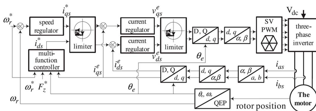
**Figure 9.** Closed-loop field-oriented control realization method. Adapted with permission from Ref. [99]. Copyright 2006 Elsevier.
