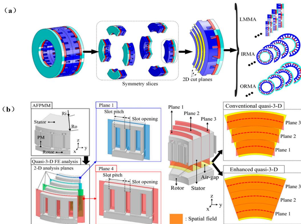
**Figure 6.** Electromagnetic modeling of FEA. (a) Diagram of converting 3D model to 2D model. Adapted with permission from Ref. [70]. Copyright 2017 John Wiley and Sons. (b) Diagram of novel quasi-3-D model. Adapted from Ref. [71].
