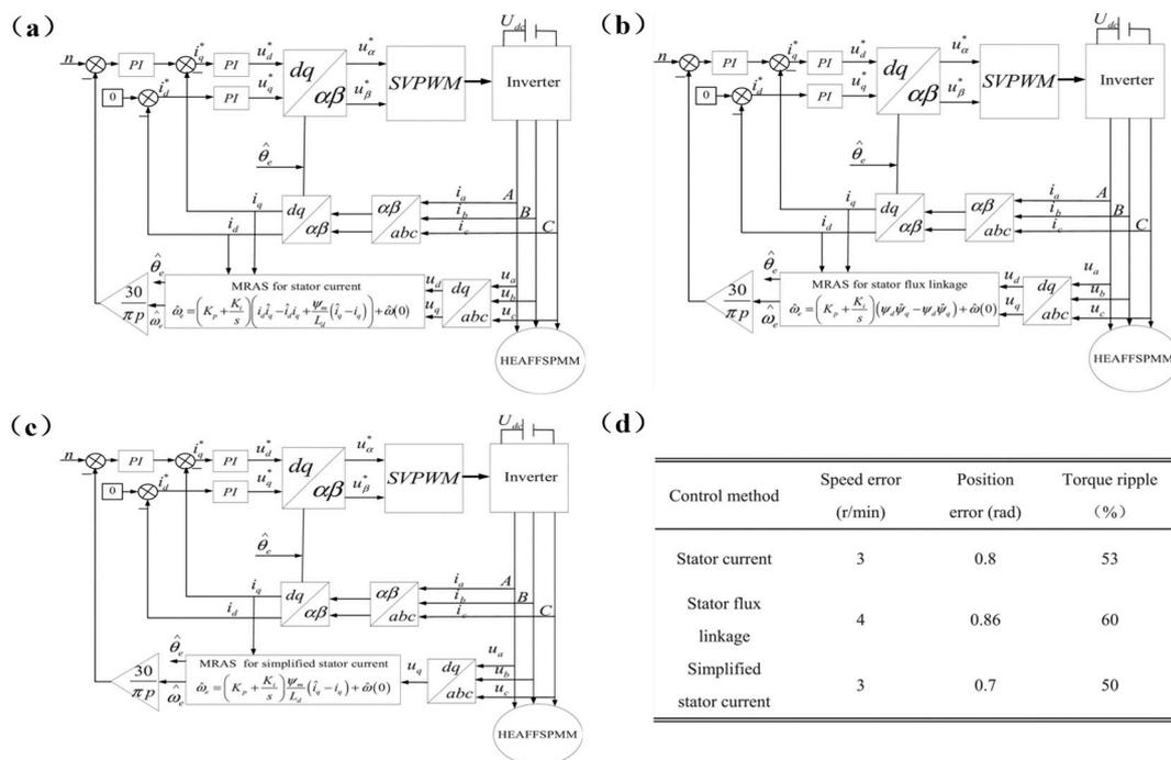
**Figure 12.** The diagrams of speed sensorless control methods based on MRAS. (a) MRAS for stator current. (b) MRAS for stator flux linkage. (c) MRAS for simplified stator current. (d) Simulation performances comparison. Adapted from Ref. [124].
