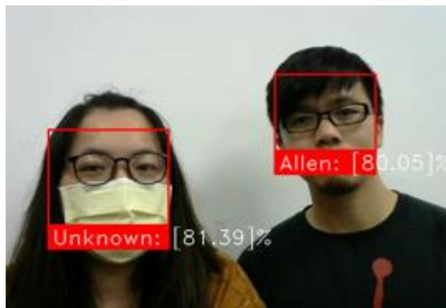
**Figure 42.** Human face detection in real time (YOLO).
