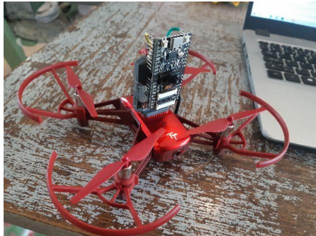
Figure 9. Our drone prototype carrying the Maix Bit.
