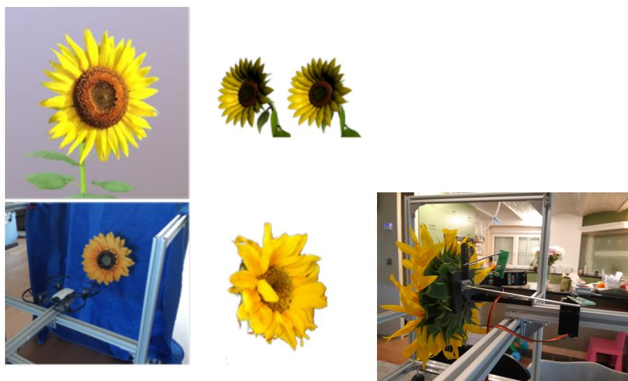
**Figure 6.** Acquisition of the training data. Top: 3D models of flowers are rendered at different angles and positions. Bottom: our chroma key set-up that is used to acquire images from both artificial (**left**) and real (**center**) sunflowers, with the drone's camera, using a 2 DoF rotator device (**right**).
