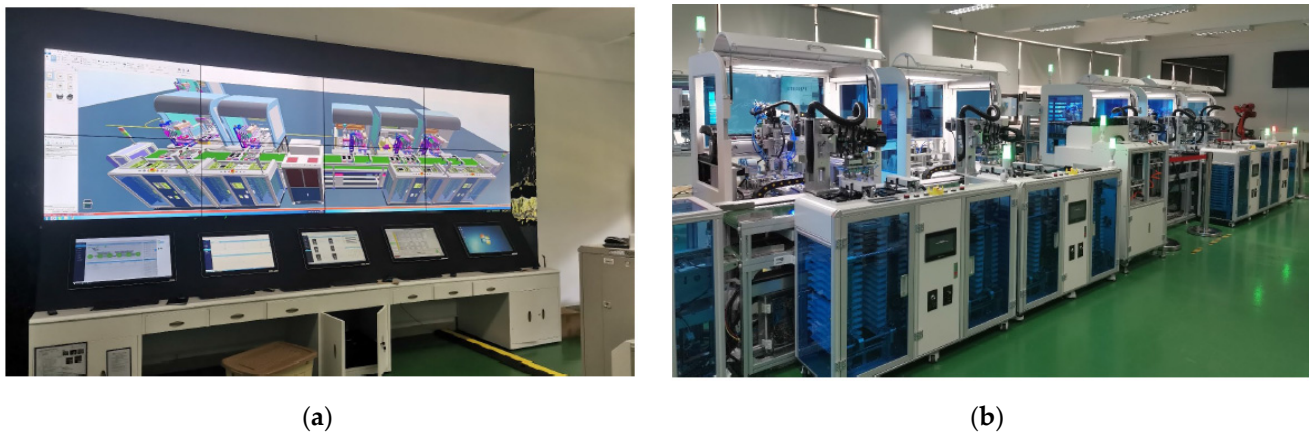
Figure 11. Mobile phone assembly line. (a) Virtual Simulation Platform. (b) Physical assembly line.
