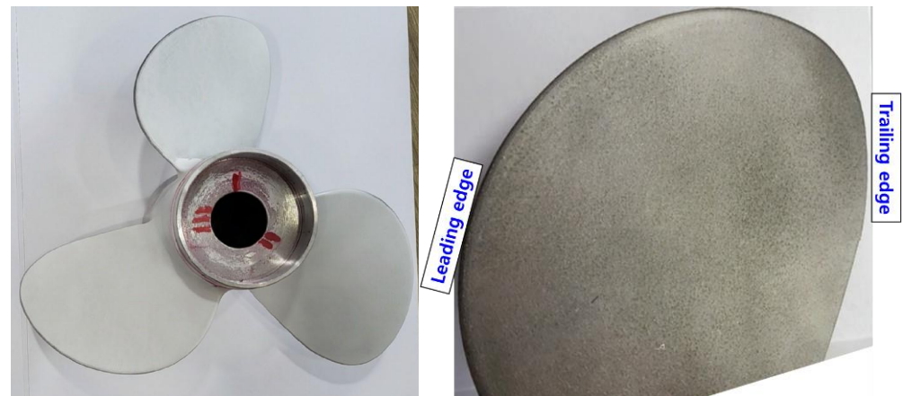
Figure 5. Photo from the liquid penetrant testing of the untreated propeller blade: (left) the suction side before sea trial and (right) one of the suction side blades after 100 h of sea trial with high-speed condition.
