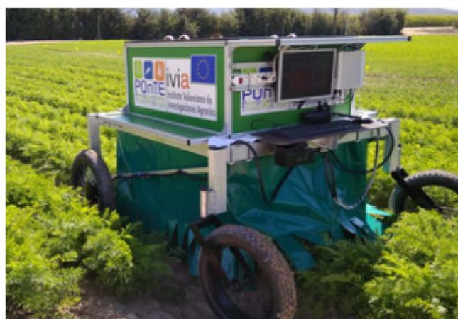
**Figure 10.** A remotely-driven RobHortic operating in a carrot field, showing the external appearance of the robot [52].
