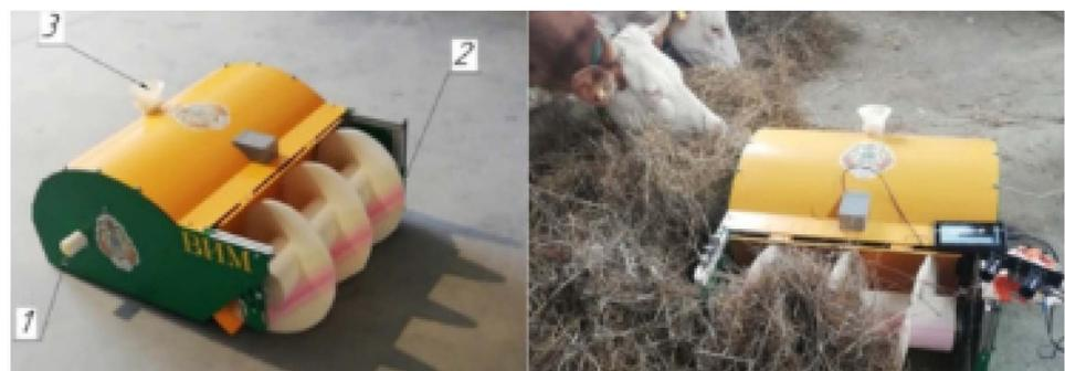
**Figure 19.** Physical analogue of a robot pusher: 1. Outlet of the feed additive dispenser; 2. Pusher auger; 3. Filler with closer [105].
