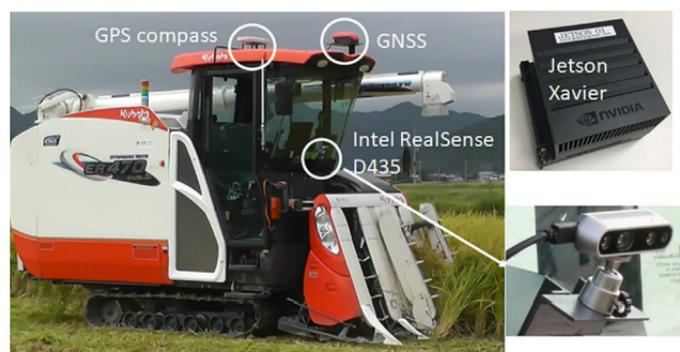
Figure 11. Robotic combine harvester and installed devices [58].
