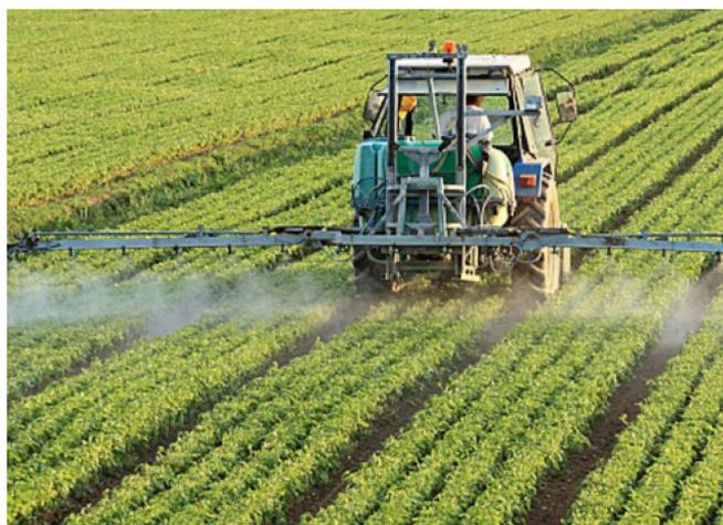
**Figure 9.** Tractor-mounted boom sprayer [50].
