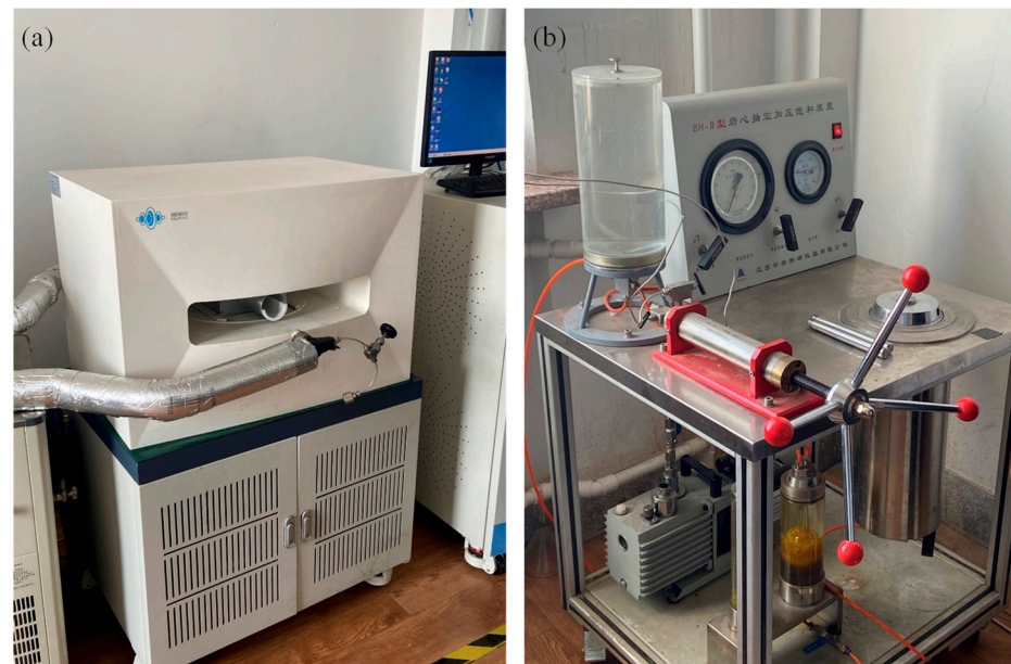
Figure 13. NMR experimental setup: (a) NMR scanner; (b) model BH-II rock core evacuation vacuum pressurization saturation device.
