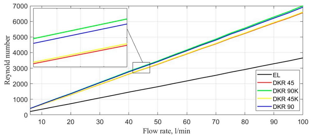
**Figure 6.** The Reynolds number of flow rate for angular fitting connections.
