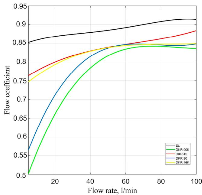
Figure 10. Flow coefficient of angular fitting connections.
