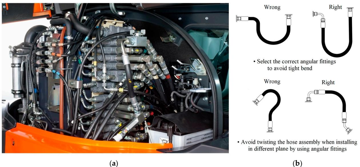
**Figure 1.** Composition of a typical hydraulic drive system: (a) part of a machine hydraulic drive system; (b) recommendation according to high-pressure hoses installation.
