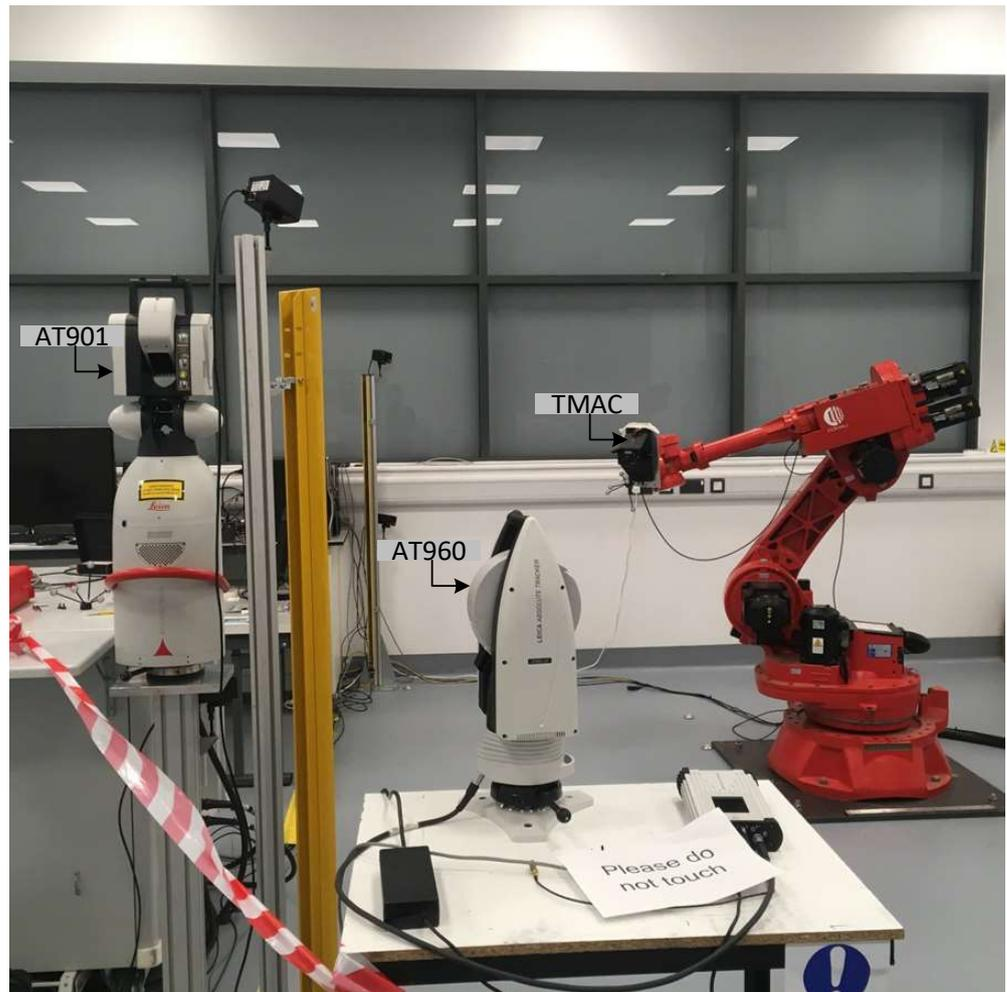
Figure 16. AT960 Leica Tracker Setup for NRTEC Verification.
