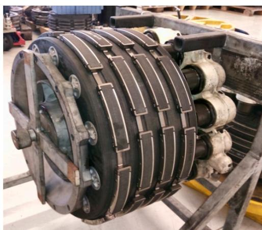
Figure 2. Multi-disc brake.
