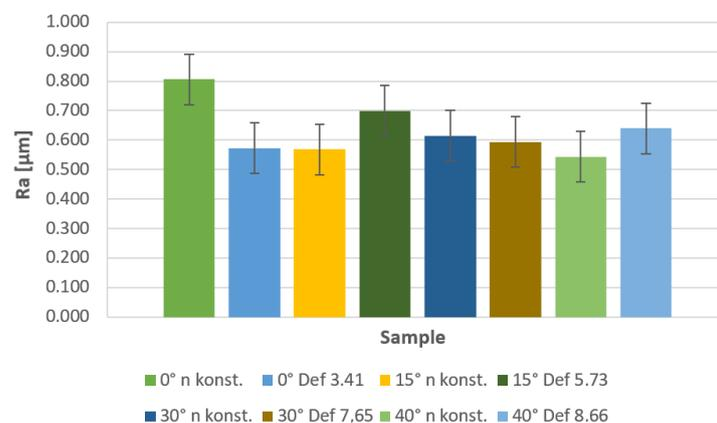
Figure 13. Comparison of roughness parameters Ra for concave parts of surfaces, non-contact method.
