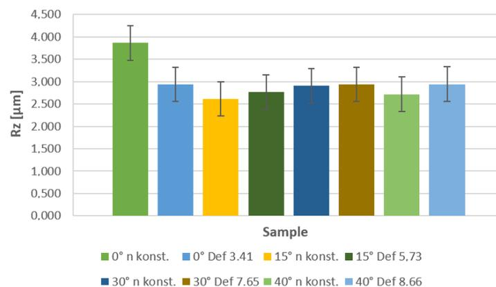
**Figure 10.** Comparison of roughness parameters Rz for concave parts of surfaces.
