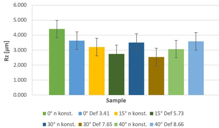
**Figure 12.** Comparison of roughness parameters Rz for convex parts of surfaces, non-contact method.
