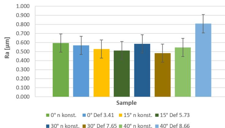
**Figure 11.** Comparison of roughness parameters Ra for convex parts of surfaces, non-contact method.
