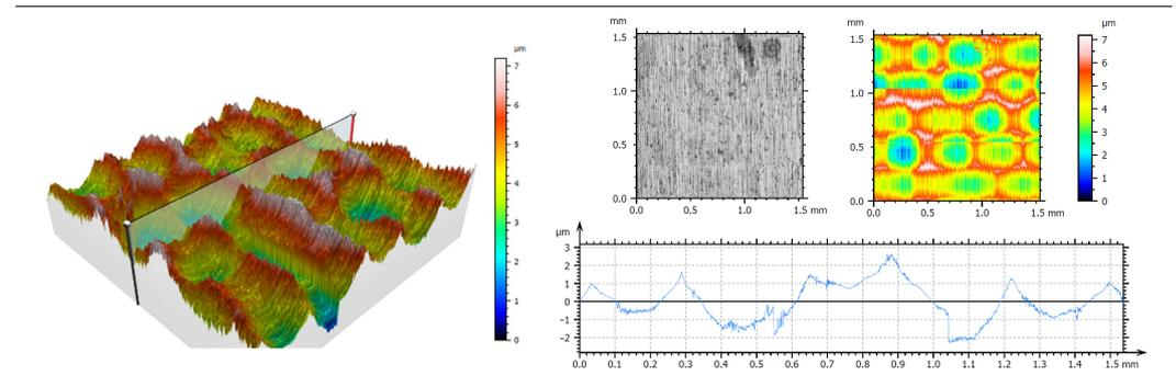
Three-dimensional view of surface texture and roughness profile at 30° n konstant
