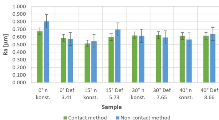
**Figure 21.** Values of the roughness parameters Ra for the concave part of the surface concerning the measurement method.
