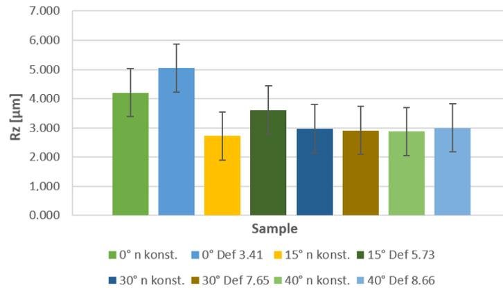
**Figure 14.** Comparison of roughness parameters Rz for concave parts of surfaces, non-contact method.
