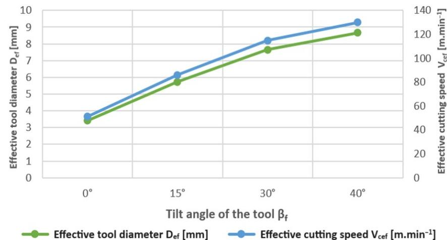
**Figure 4.** Dependence of the effective tool diameter  $d_{ef}$  and the effective cutting speed  $v_{cef}$  on the position of the tool axis  $\beta_f$ .
