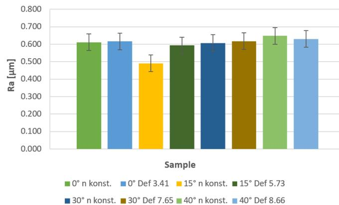
**Figure 7.** Comparison of roughness parameters Ra for convex parts of surfaces.
