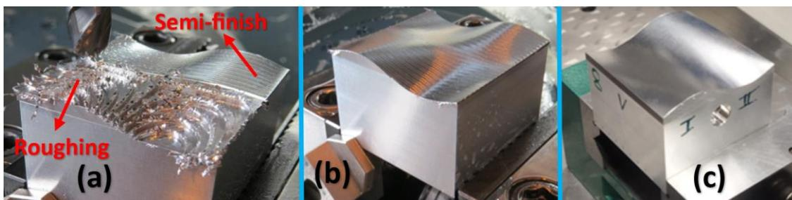
Figure 3. Visual comparison of the real production (a) roughing, (b) semi-finish, and (c) after finish.
