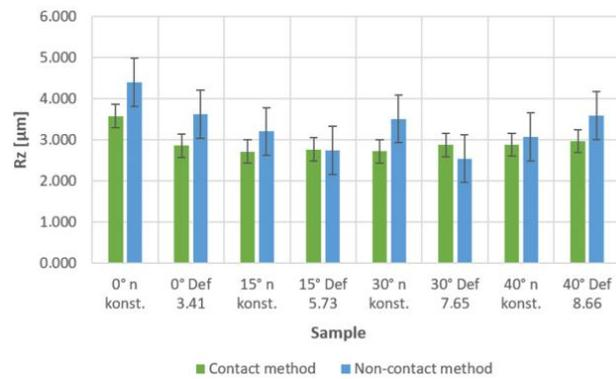
**Figure 20.** Values of the roughness parameters Rz for the convex part of the surface concerning the measurement method.
