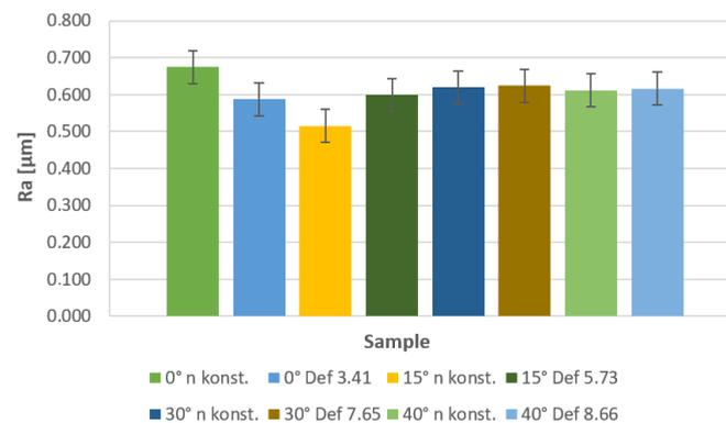
**Figure 9.** Comparison of roughness parameters Ra for concave parts of surfaces.**Table 11.** Measured values of roughness Rz [ $\mu\text{m}$ ] for the concave part of the surface by contact method.
