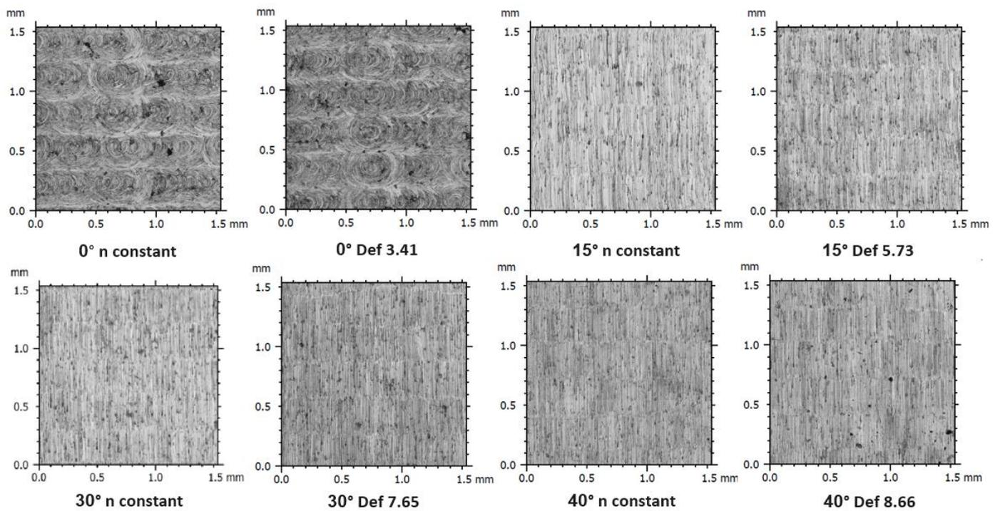
**Figure 16.** Two-dimensional topography of the concave parts of the surfaces according to the inclination of the tool.
