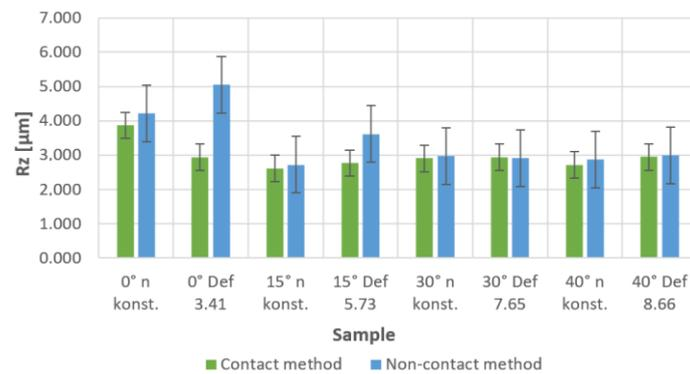
**Figure 22.** Values of the roughness parameters Rz for the concave part of the surface concerning the measurement method.
