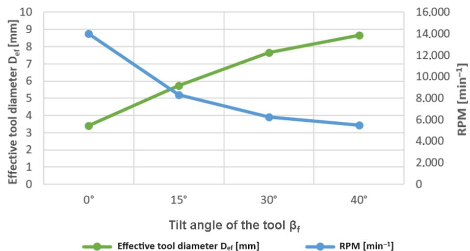
**Figure 5.** Dependence of the effective tool diameter  $d_{ef}$  and revolutions  $n$  on the position of the tool axis  $\beta_f$ .
