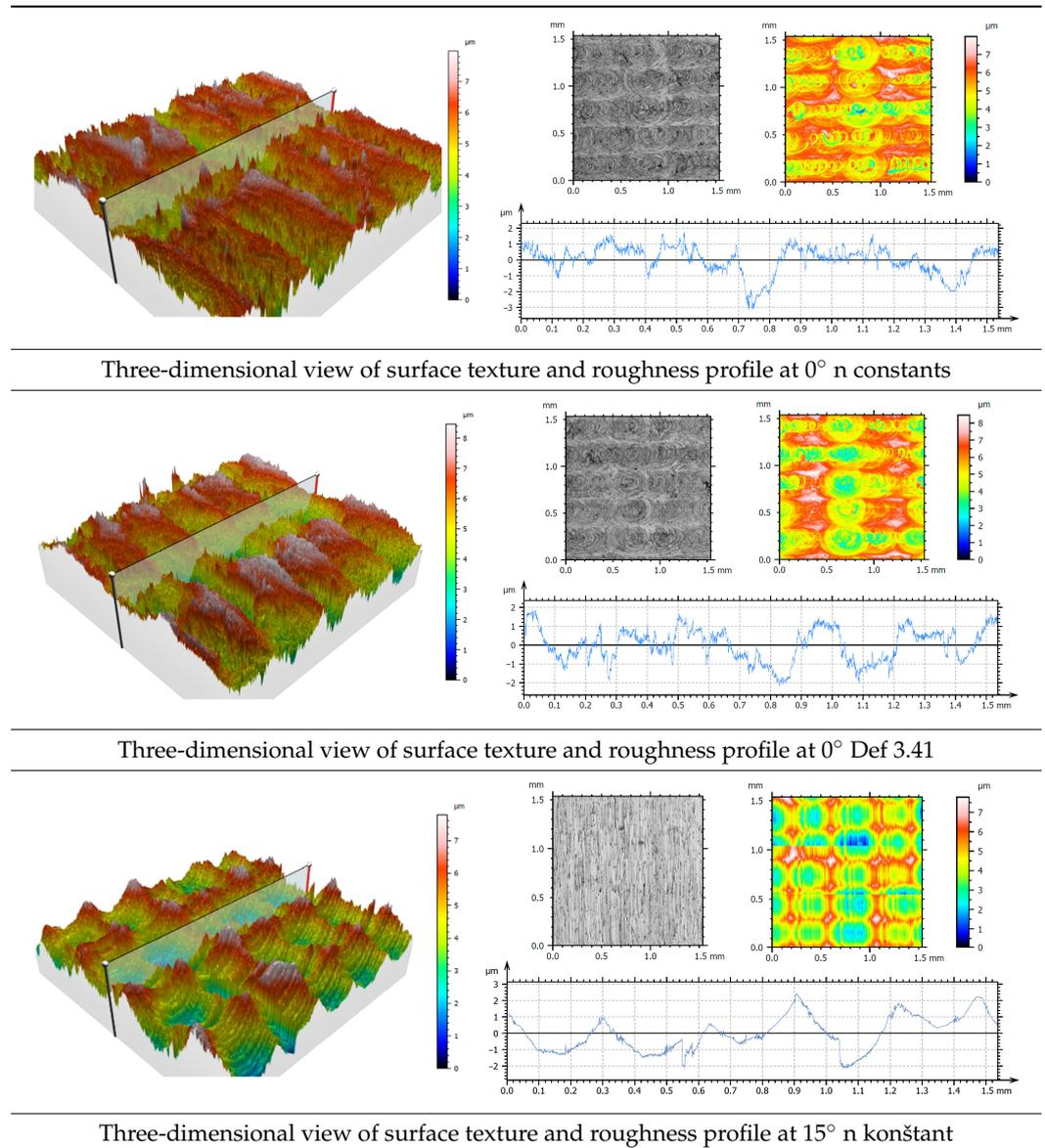
Three-dimensional view of surface texture and roughness profile at 0° n constants
