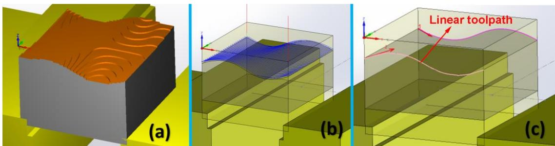
Figure 2. Visual comparison of the operation used (a) roughing (b) semi-finish, and (c) finish operation.
