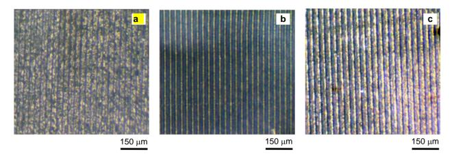
**Figure 8.** Veeco Dektak Stylus Profilometry 2D for LDPE films imprinted with (a) no heat; (b) 1.2 kW and (c) 1.6 kW.
