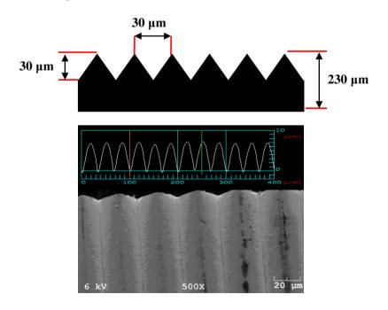
A closed-loop flexible belt mold was prepared from electroformed nickel alloy sheets containing sawtooth type features, 30  $\mu$ m in height and pitch, as shown in Figure 6. Specifically, strips of nickel alloy sheets were assembled together using heat tolerant Kapton® polyimide tape. The completed belt mold is approximately 10 cm wide, 50 cm long, and 250  $\mu$ m thick. It was finally installed onto the modified rolling mill through the upper roller (Figure 4b).
