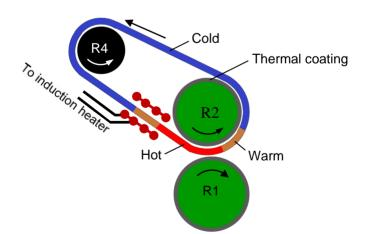
Figure 3. Induction heating of belt mold.
