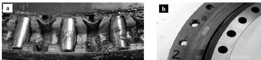
Figure 12. Slew bearing damage: (a) A view of damaged rollers in the axial plane; (b) Outer raceway damage.
